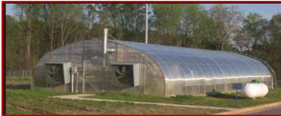
Fig. 1.3.6 Quonset Type Greenhouse
