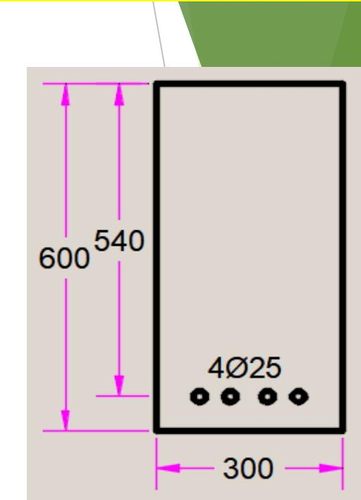
$$As_{min} = \frac{1.4}{f_y} b_w d = \frac{1.4}{420} \times 300 \times 540 = 540 \text{ mm}^2 \quad (OK)$$
