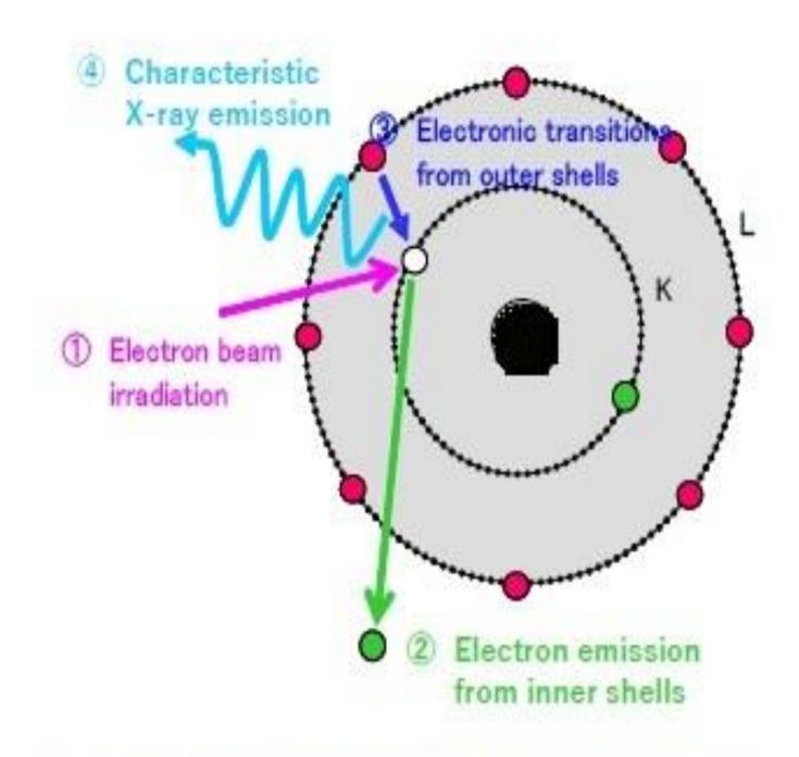
Fig. 2. Mechanism of electron and characteristic X-ray emission resulting from electron irradiation.
