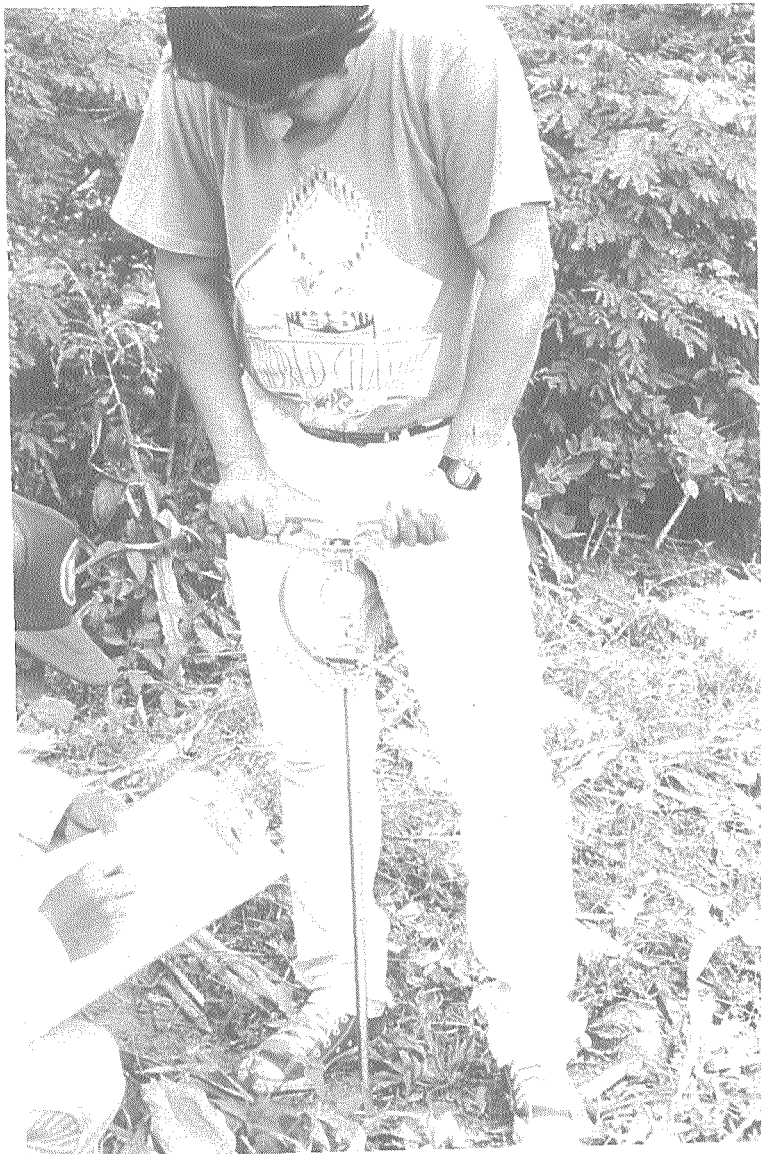
Figure 4.5 Measuring soil resistance with cone penetrometer
