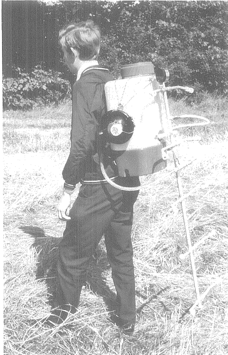
Figure 2.1 Vibration type time recorder attached to a manually operated sprayer
