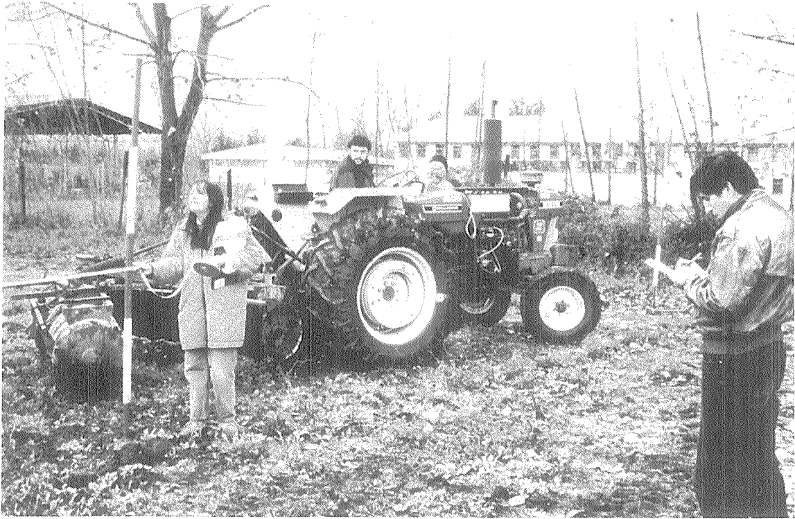
Figure 4.22 Field measurement of forward speed, wheelslip and turning time
