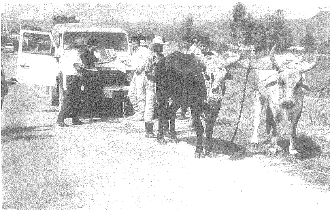
Figure 4.17 Measurement of instantaneous maximum force of oxen using a vehicle as an anchor
