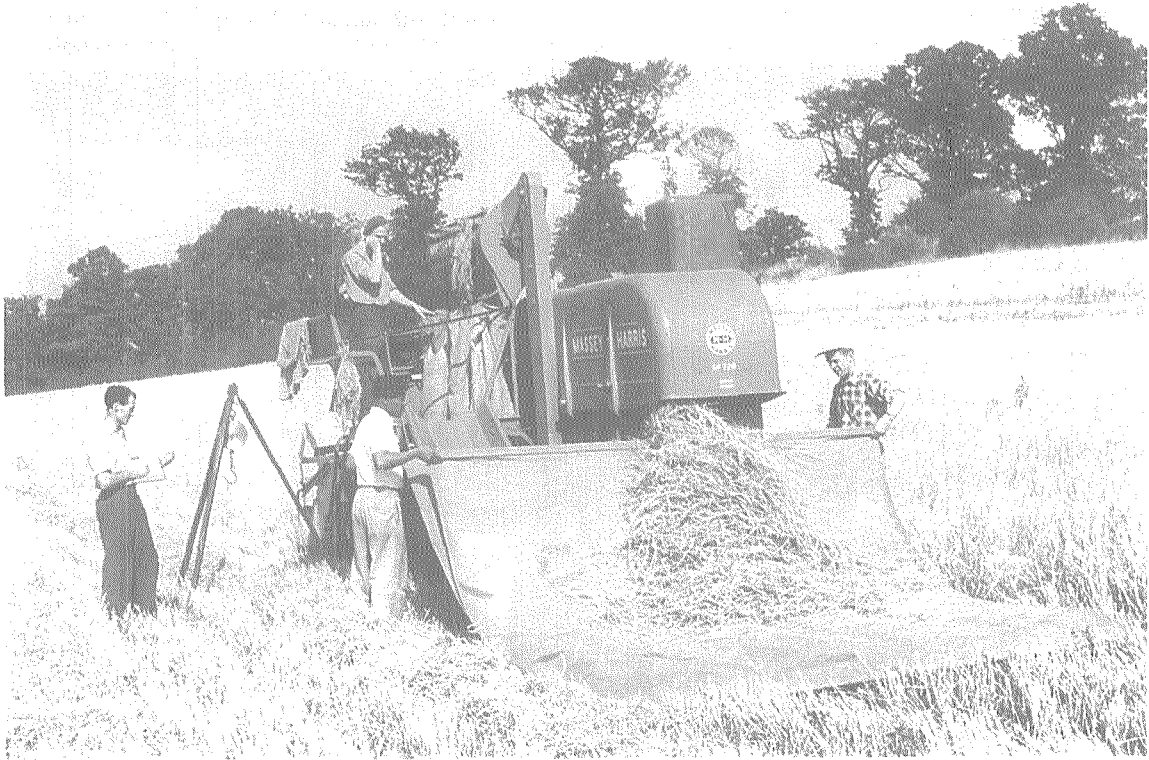
Figure 4.43 Collection of combine straw shaker and sieve outputs during a test run
