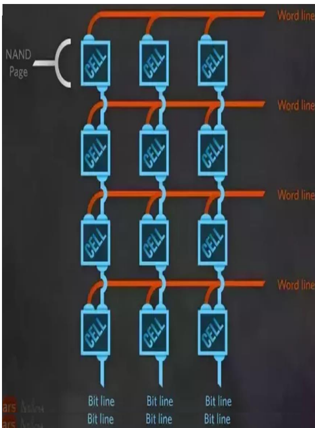
Figure 5.9 Flash Memory Structure
