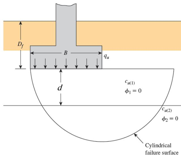
**Fig. 3.10** Footing on layered clays
