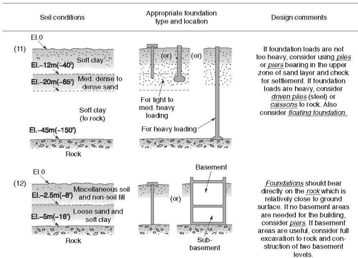
Fig. 1.2 Illustrations relating soil conditions and appropriate foundation types
