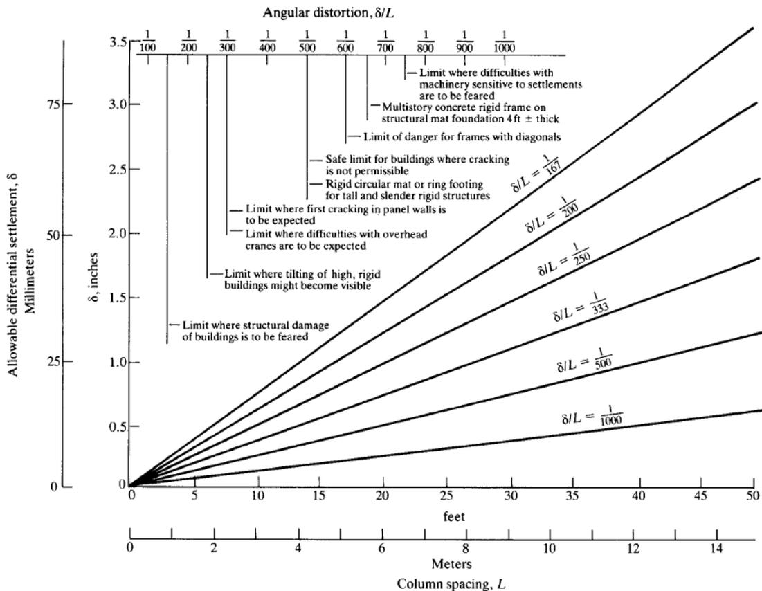
**Fig. 4.27 Tolerable settlements for buildings. (Bjerrum, 1963; Navy, 1982)**
