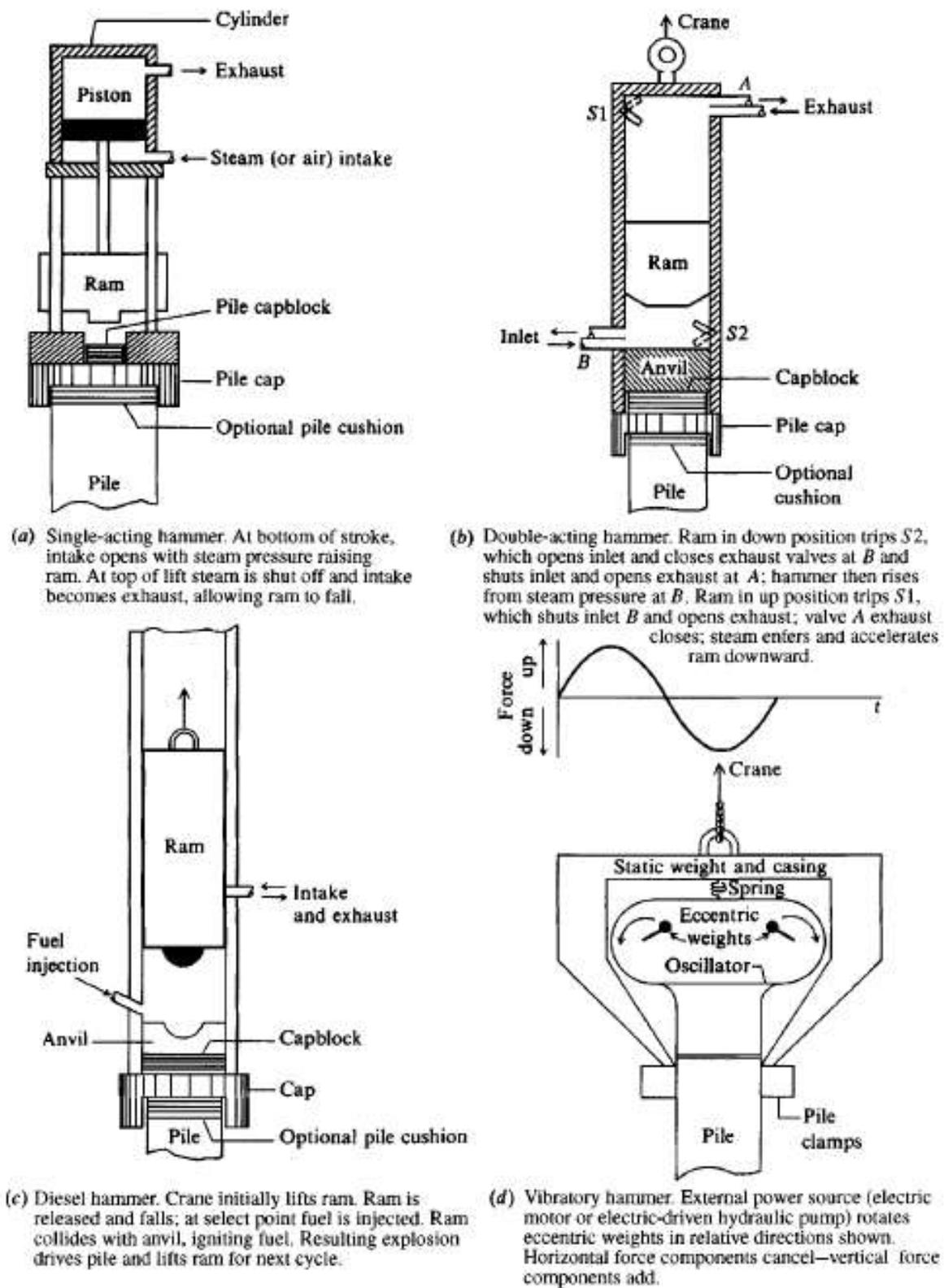
Fig. 8.14 Schematics of several pile hammers.
