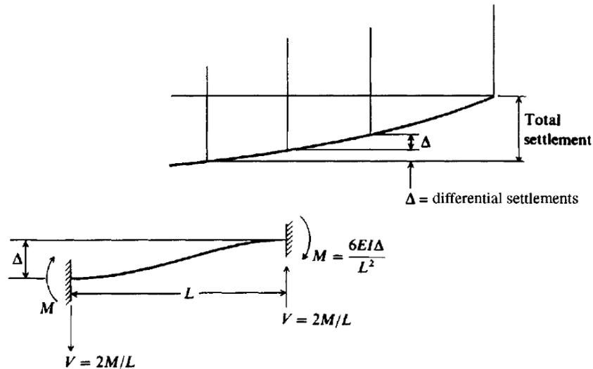
**Fig. 7.2** Reduction of bending moments in superstructure by using mat foundation. Bending moment  $M$  is based on differential settlement between columns and not on total settlement.
