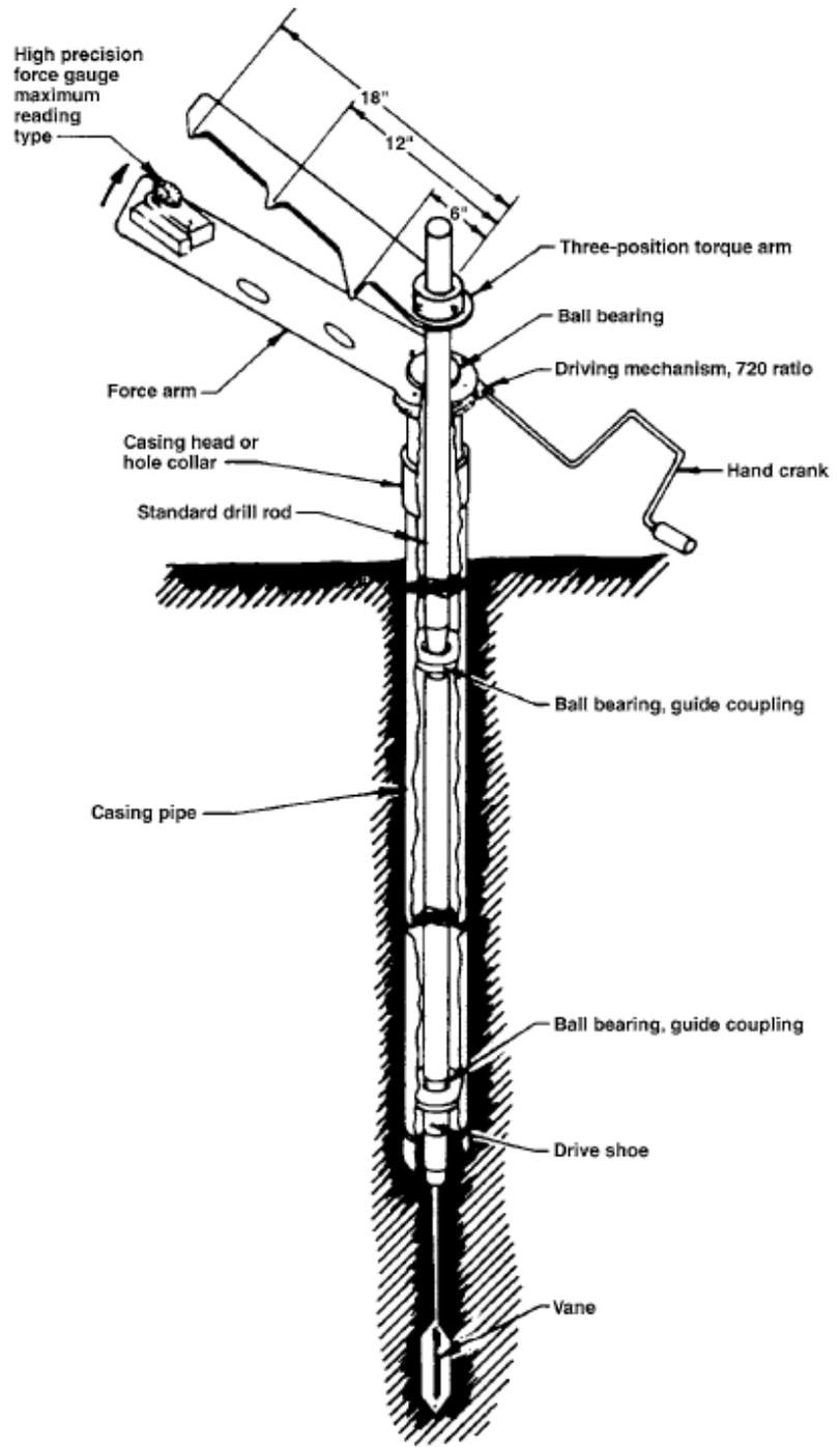
Fig. 2.18 Diagram illustrating the field vane test.
