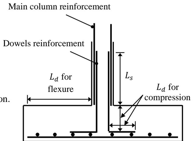
Fig. 5.5 Development lengths and lap splices
