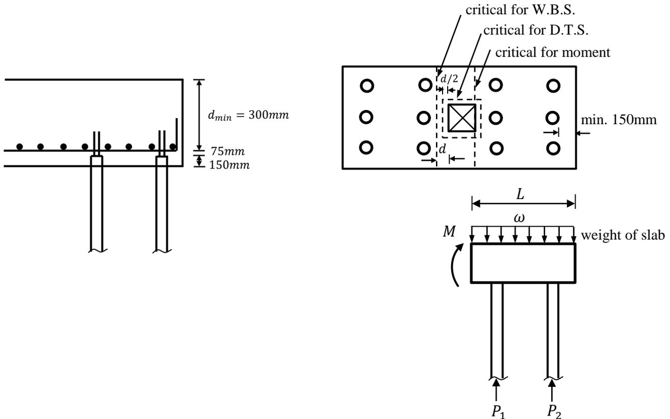
**Fig. 9.6** Critical pile cap locations for shear, moment, and bond according to ACI-318.
