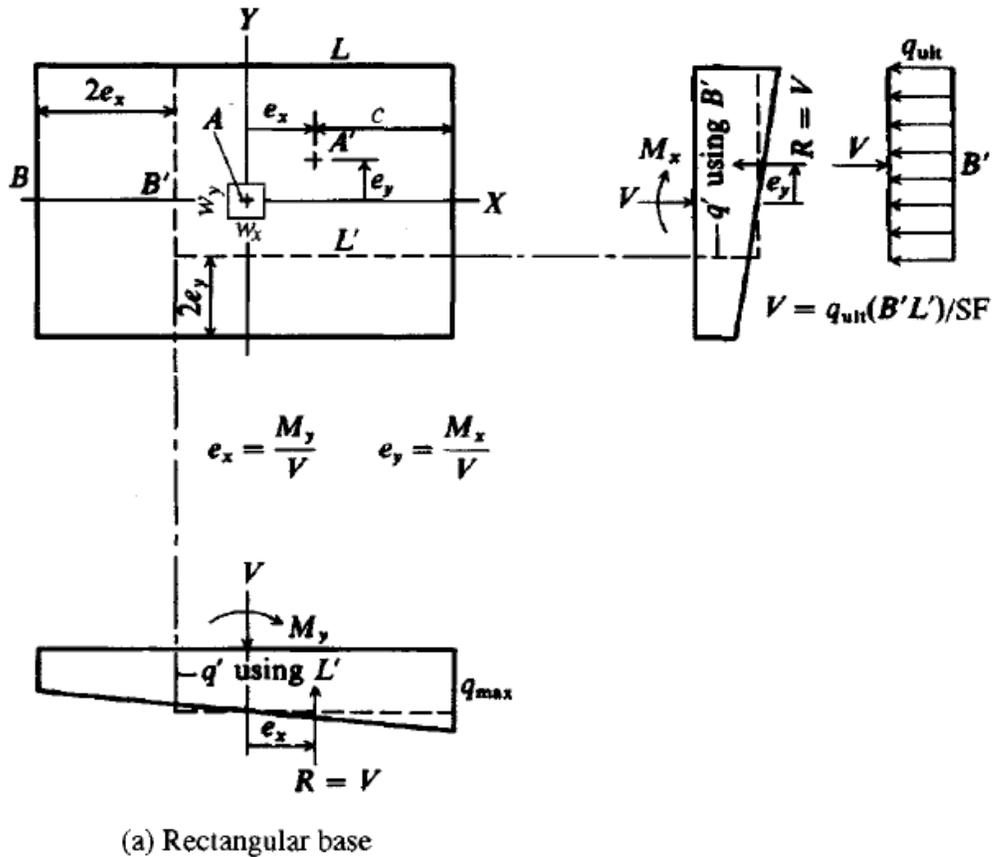
**Fig. 3.8** Method of computing effective footing dimensions when footing is eccentrically loaded for rectangular footing
