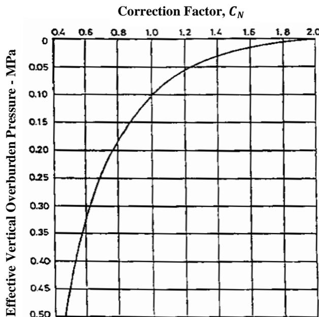
**Fig. 2.14** Chart for correction of  $N$ -values for influence of overburden pressure
