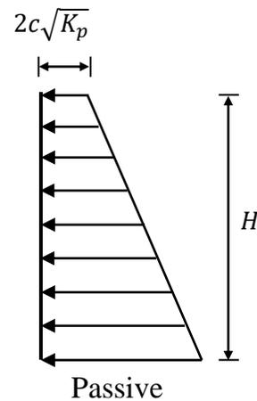
**Fig. 10.5** Passive lateral earth pressure distribution for a  $(c - \phi)$  soil
