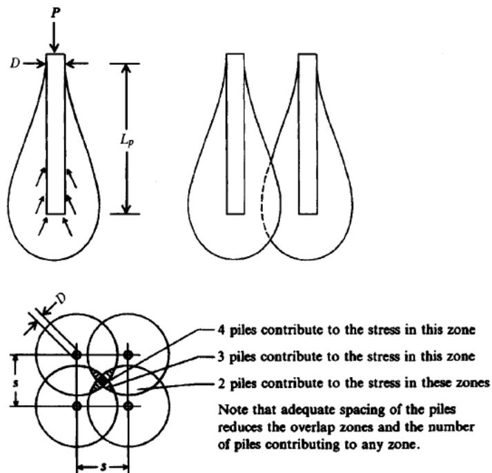
Fig. 9.2 Stresses surrounding a friction pile and the summing effects of a pile group.
