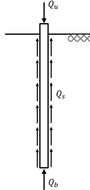
Fig. 8.3 Components of pile carrying capacity
