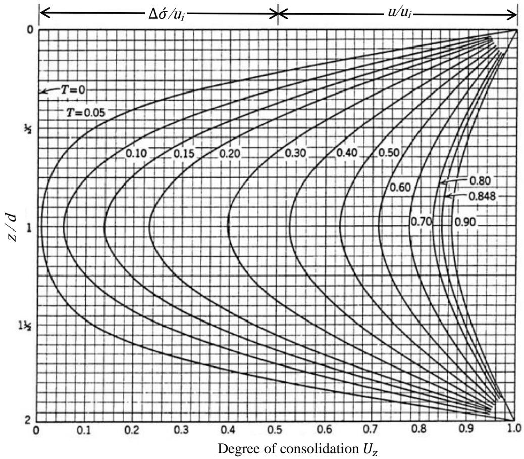
Fig. 4.22 Variation of  $U_z$  with  $T_v$  and  $z/d$
