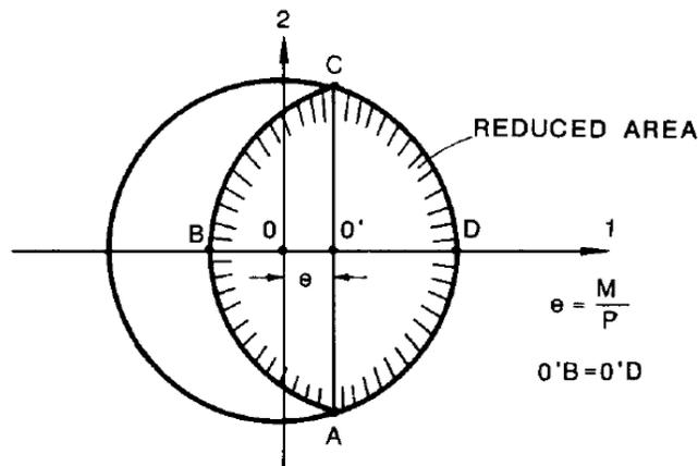
Fig. 3.9 Reduced (effective) area for circular footing
