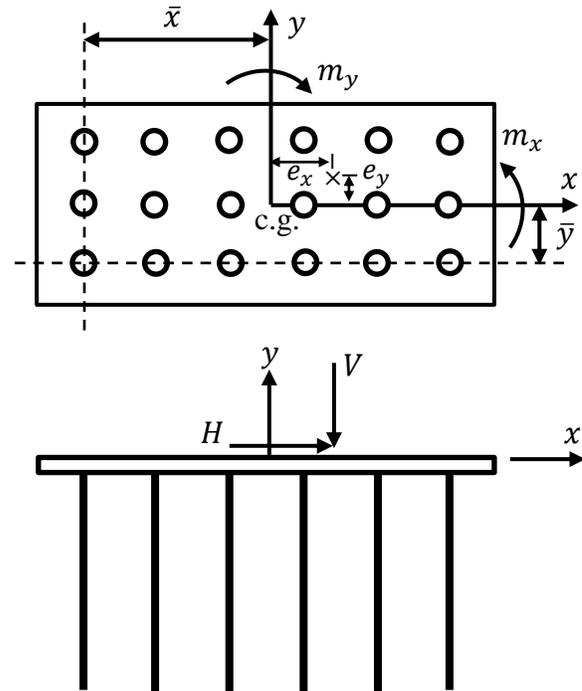
**Fig. 9.5** An eccentric loading on group of vertical piles
