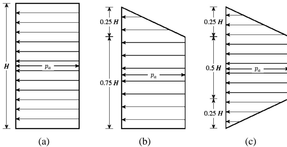
Fig. 12.9 Apparent-pressure envelope for (a) cuts in sand, (b) cuts in soft to medium stiff clay, and (c) cuts in stiff clay
