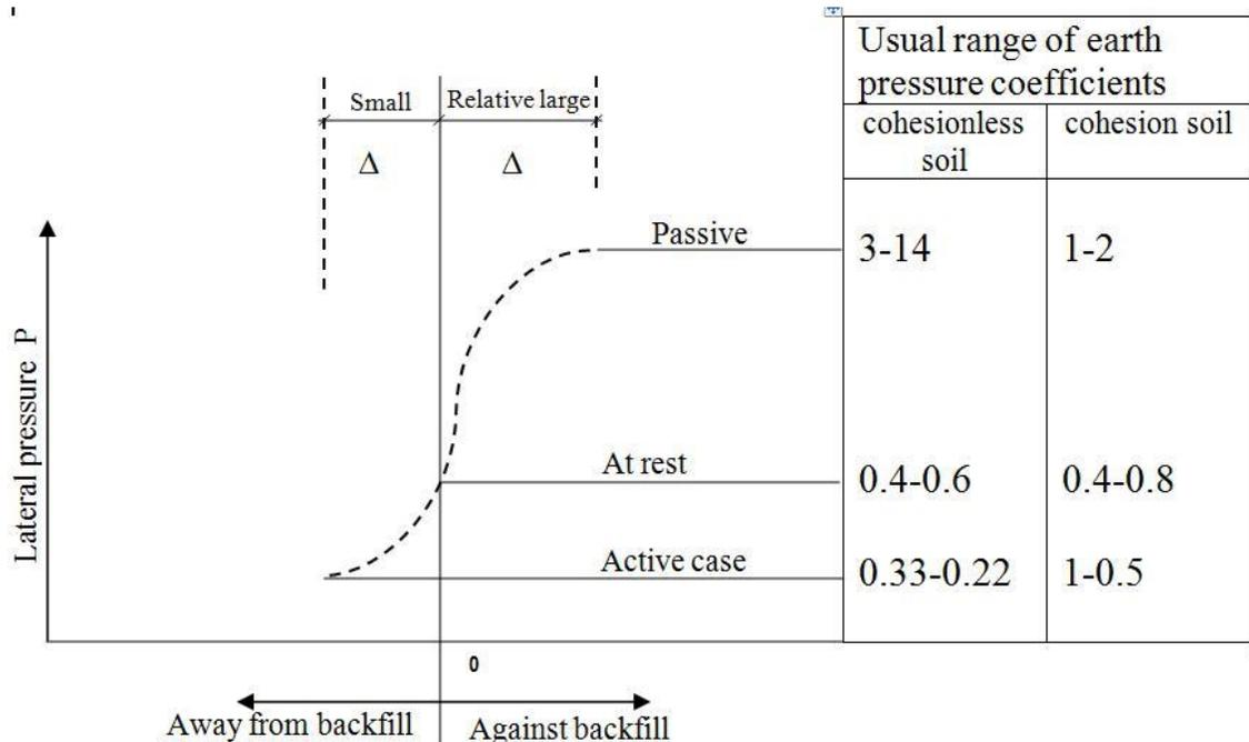
**Fig. 10.1** Illustration of active and passive pressures with usual range of values for cohesionless and cohesive soils
