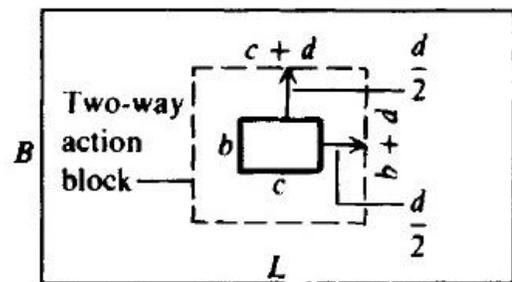
Fig. 5.1 Critical section for two-way action (punching) shear
