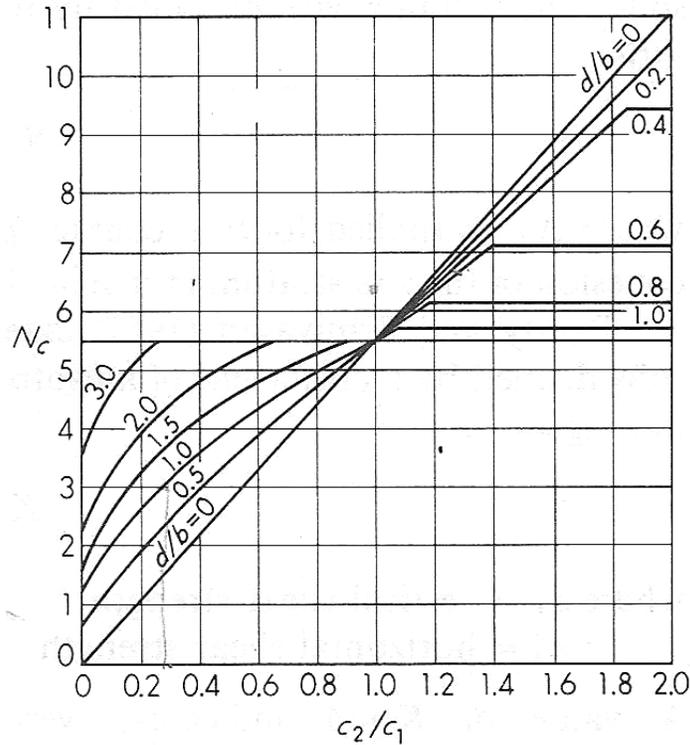
Fig. 3.11 Bearing capacity factor  $N_c$  for a footing on layered clays
