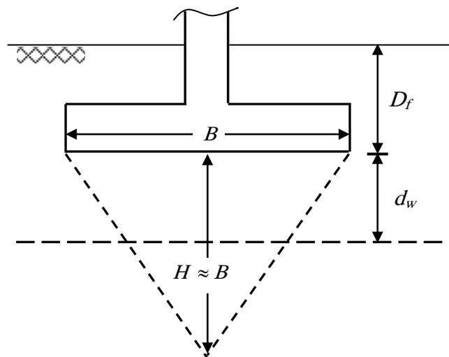
Fig. 3.14 Correction of  $(q_a)_{net}$  for water table
