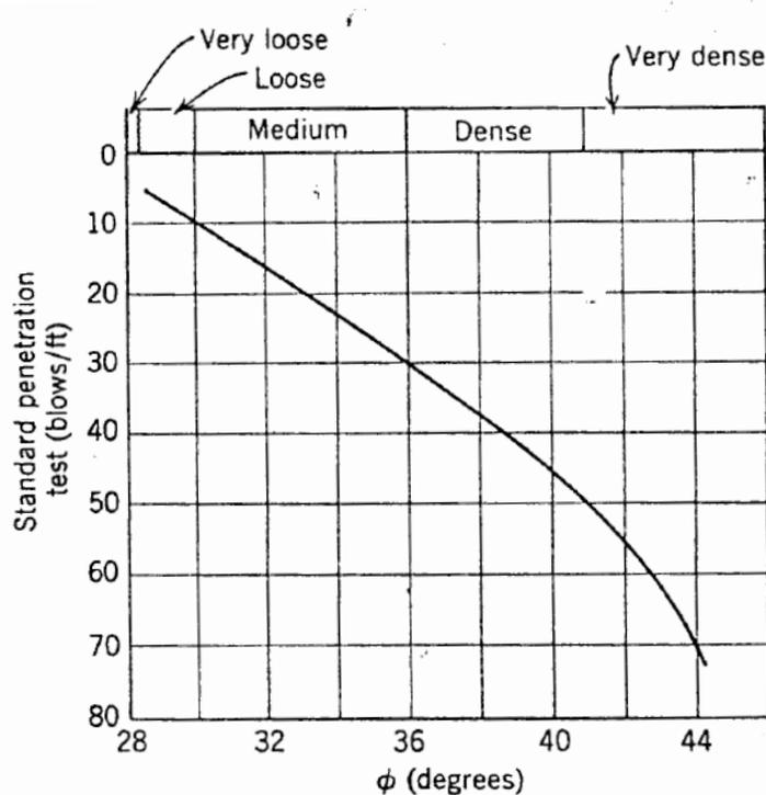
**Fig. 8.10** Correlation between friction angle and penetration resistance
