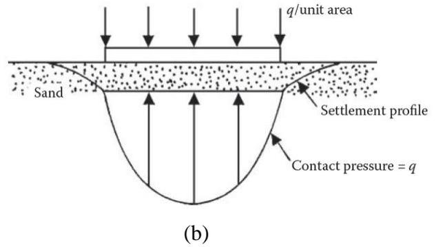
**Fig. 4.2** Flexible (a) and rigid (b) foundations on sand
