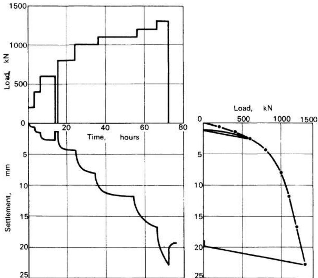
**Fig. 8.13** Method of presenting the result of a load test, giving plottings of load and settlement versus time and of load versus the maximum settlement at each stage of loading
