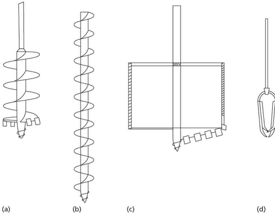
Fig. 2.2 (a) Short-flight auger, (b) continuous-flight auger, (c) bucket auger, and (d) Iwan (hand) auger.
