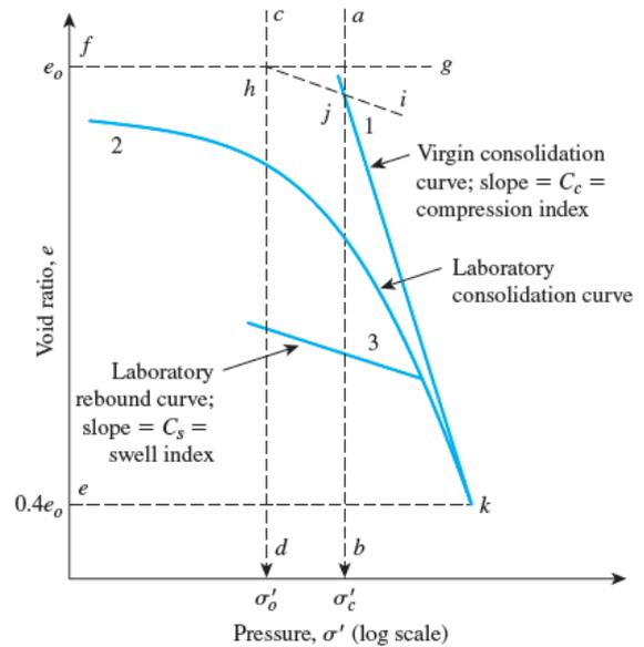
**Fig. 4.17** Consolidation characteristics of overconsolidated consolidated clay of low to medium sensitivity
