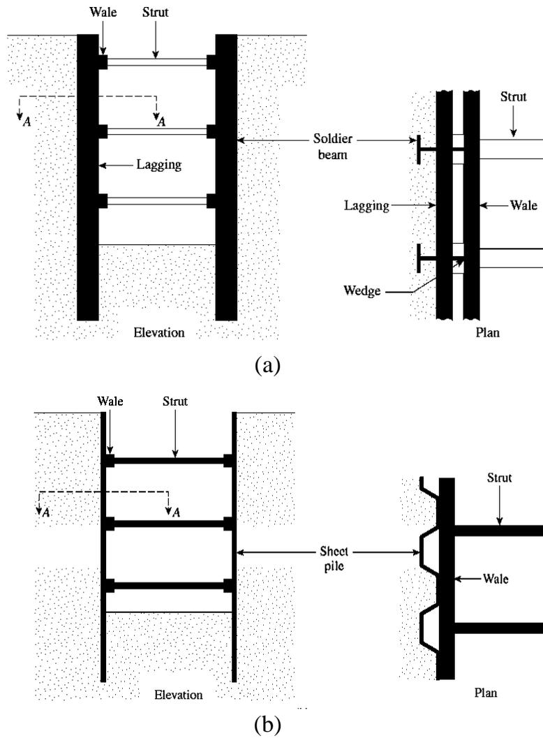
Fig. 12.8 Types of braced cut: (a) use of soldier beams; (b) use of sheet piles
