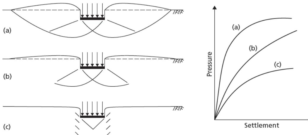
**Fig. 3.1** Modes of failure: (a) general shear, (b) local shear, and (c) punching shear.
