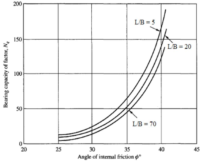
Fig. 8.5 Berezantsev's bearing capacity factor,  $N'_q$
