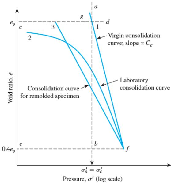
**Fig. 4.16** Consolidation characteristics of normally consolidated clay of low to medium sensitivity
