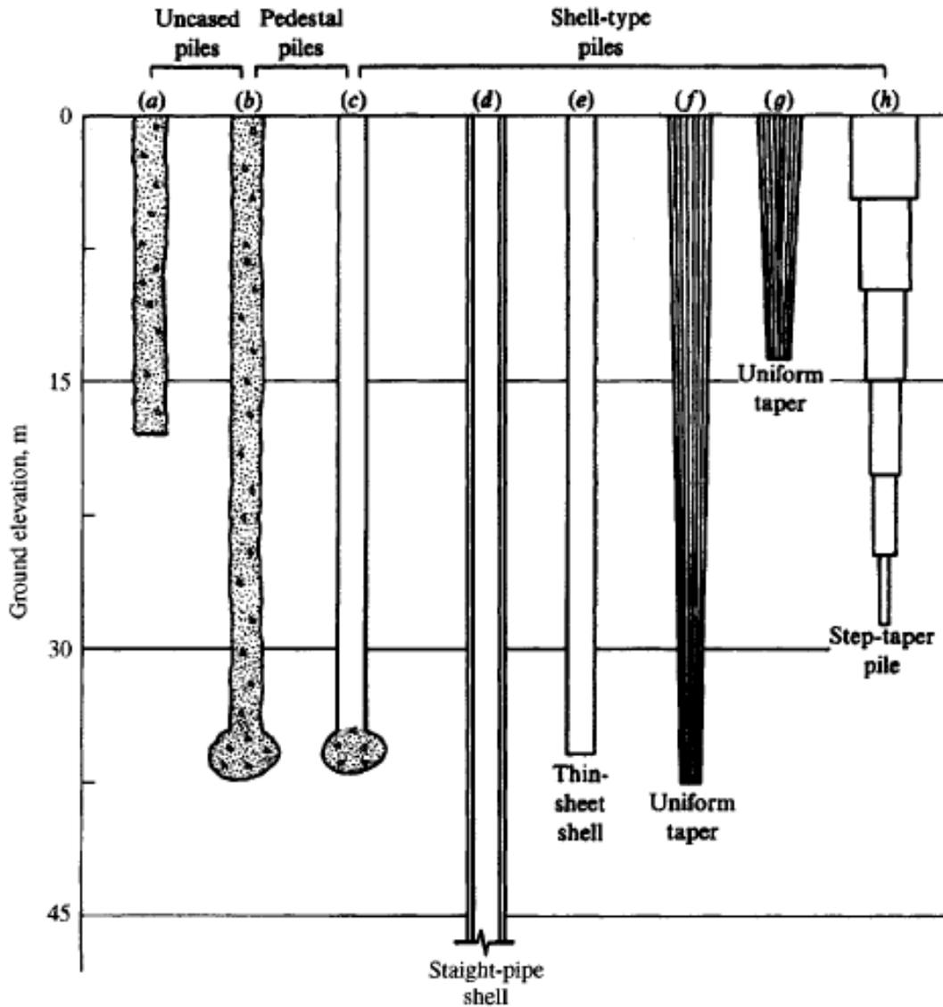
**Fig. 8.2** Some common types of cast-in-place (patented) piles: (a) Commonly used uncased pile; (b) Franki uncased pedestal pile; (c) Franki cased pedestal pile; (d) welded or seamless pipe; (e) Western cased pile; (f) Union or Monotube pile; (g) Raymond standard; (h) Raymond step-taper pile. Depths shown indicate usual ranges for the various piles. Current literature from the various foundation equipment companies should be consulted for design data.
