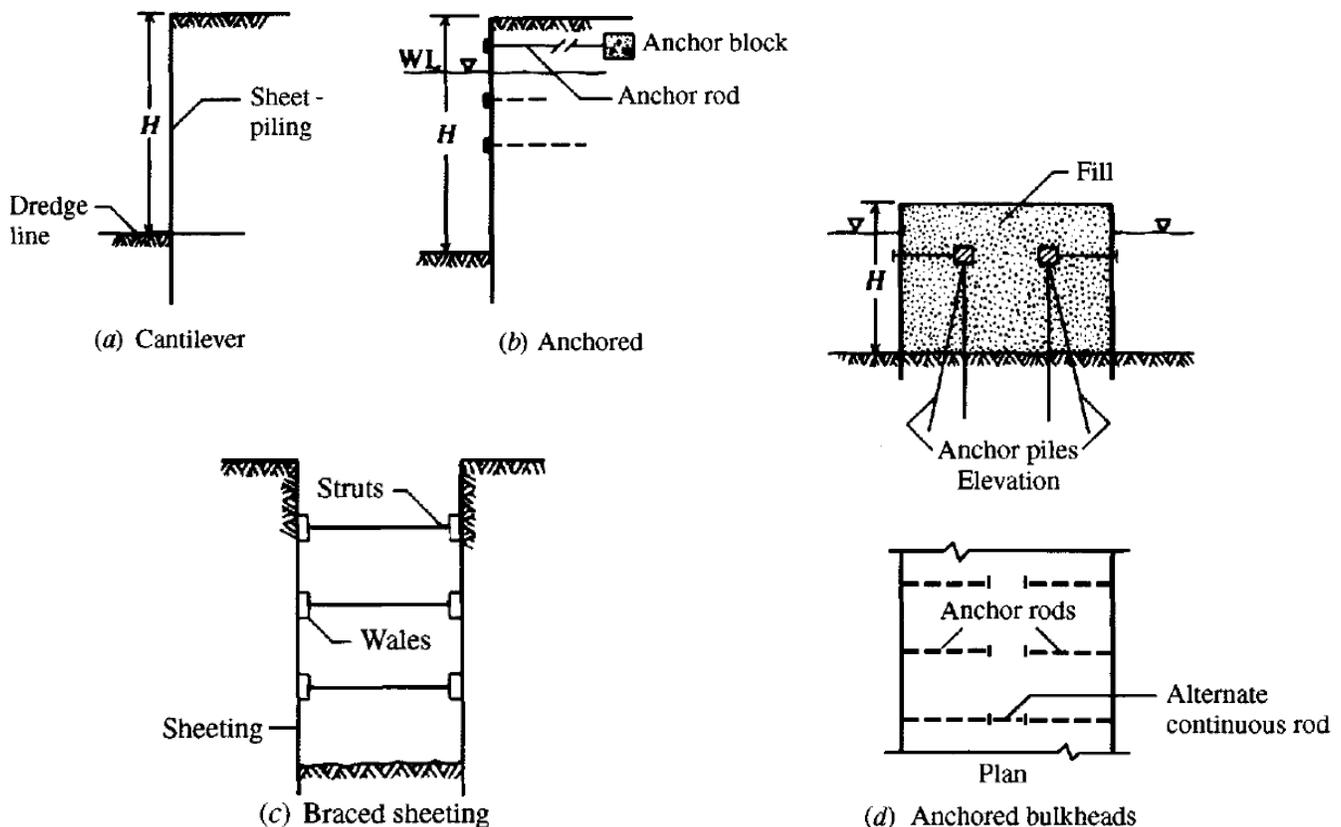
Fig. 12.1 Sheet-pile structures
