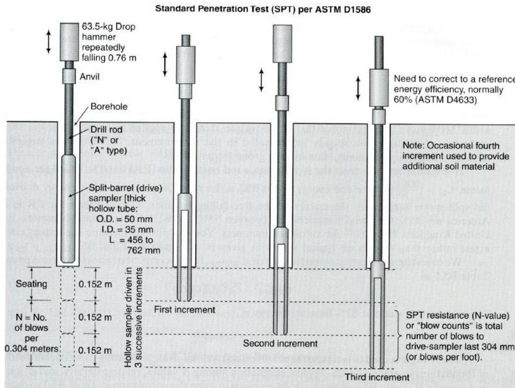
**Fig. 2.13** Driving sequence in an SPT
