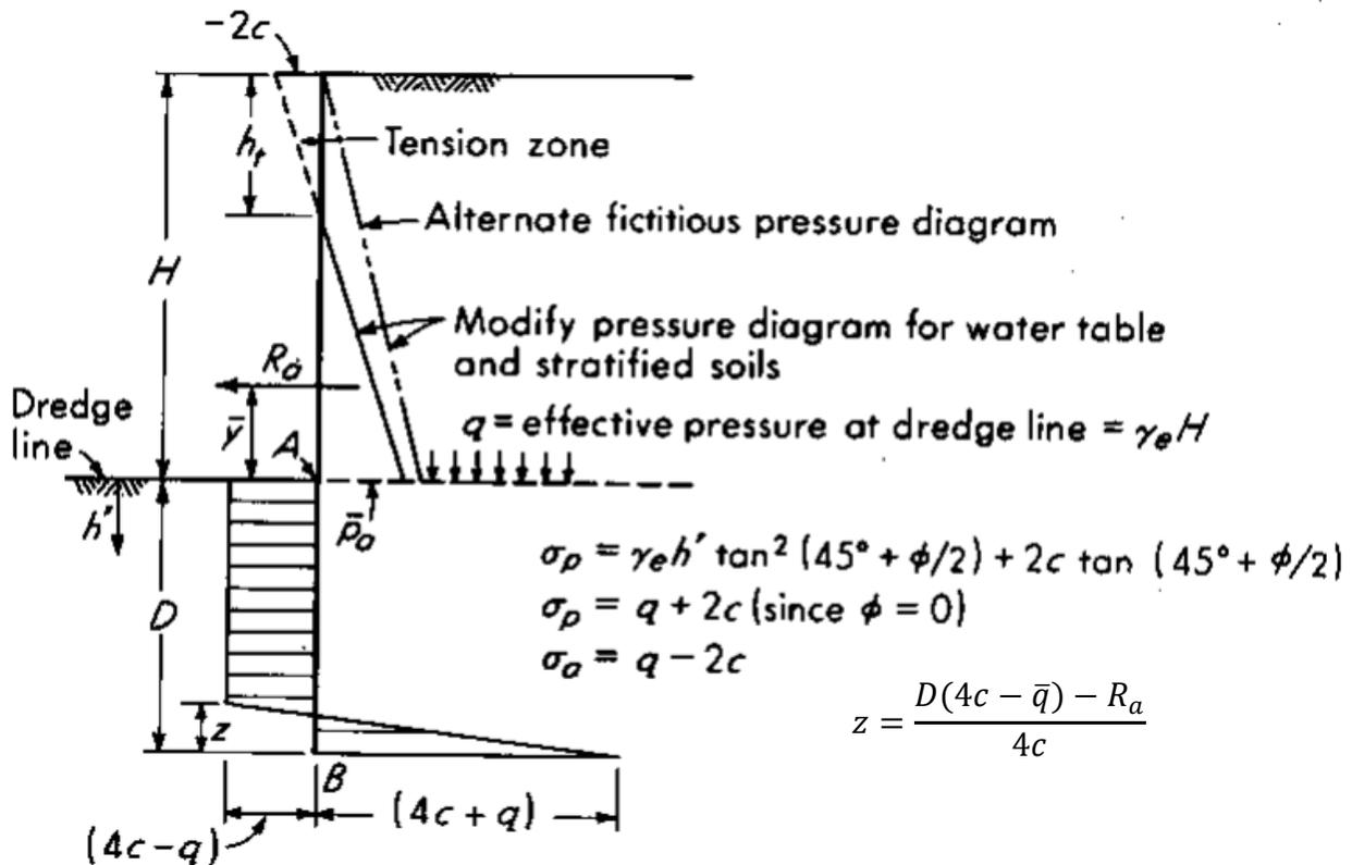
Fig. 12.4 Sheetpiling in cohesive soil. The undrained shear strength ( $\phi = 0$ ) case shown is conservative.
