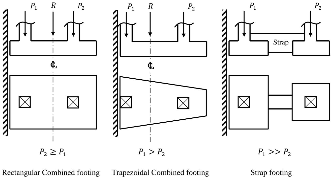
Fig. 6.2 Possible types of combined footing
