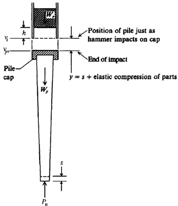
**Fig. 8.15** Significance of certain terms used in the dynamic pile-driving equations.
