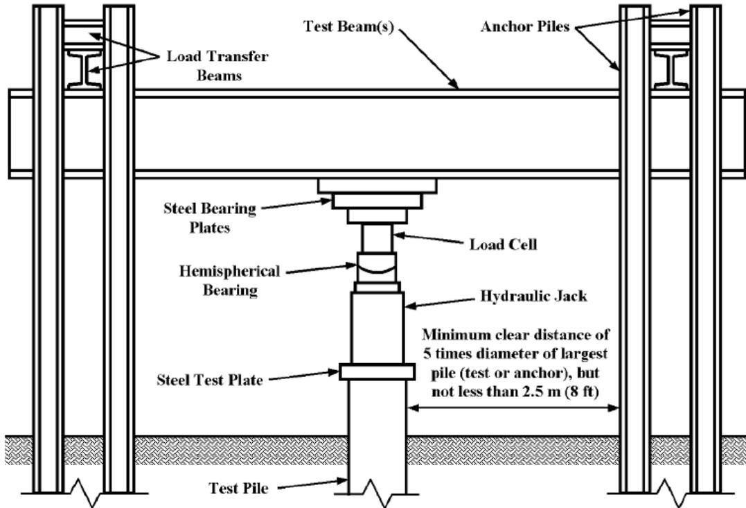
Fig. 8.11 Schematic of hydraulic jack acting against anchored reaction frame
