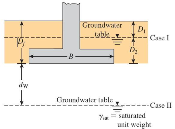
**Fig. 3.6** Modification of bearing capacity equations for water table
