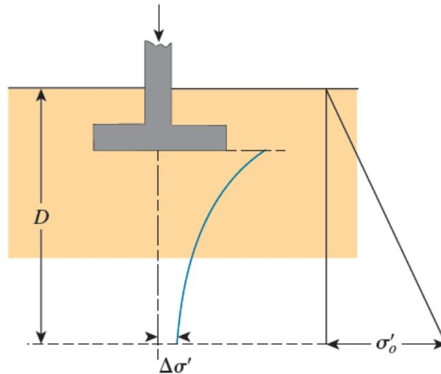
Fig. 2.12 Determination of the minimum depth of boring
