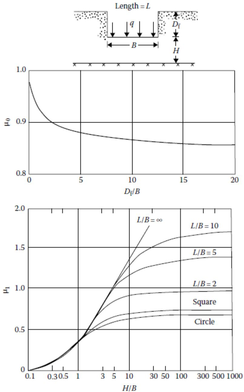
Fig. 4.13 Coefficients for vertical displacement of foundations on saturated clays
