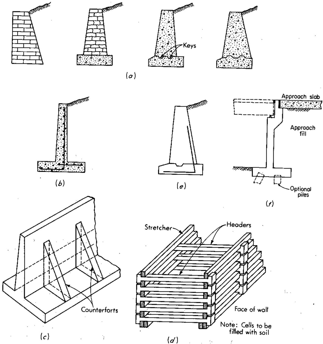
**Fig. 11.1** Types of retaining walls. (a) Gravity walls of stone masonry, brick, or plain concrete. Weight provides overturning and sliding stability; (b) cantilever wall; (c) counterfort, or buttressed wall. If backfill covers counterforts, the wall is termed a counterfort; (d) crib wall; (e) semigravity wall (small amount of steel reinforcement is used); (f) bridge abutment.
