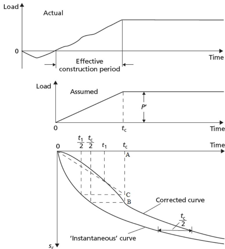
**Fig. 4.24** Correction for construction period
