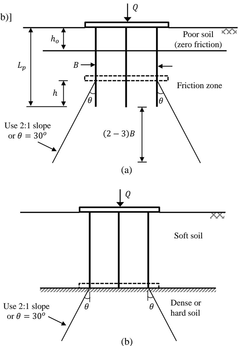
**Fig. 9.4** Simplified computation of soil stresses beneath a pile group; (a) friction piles, (b) point-bearing piles
