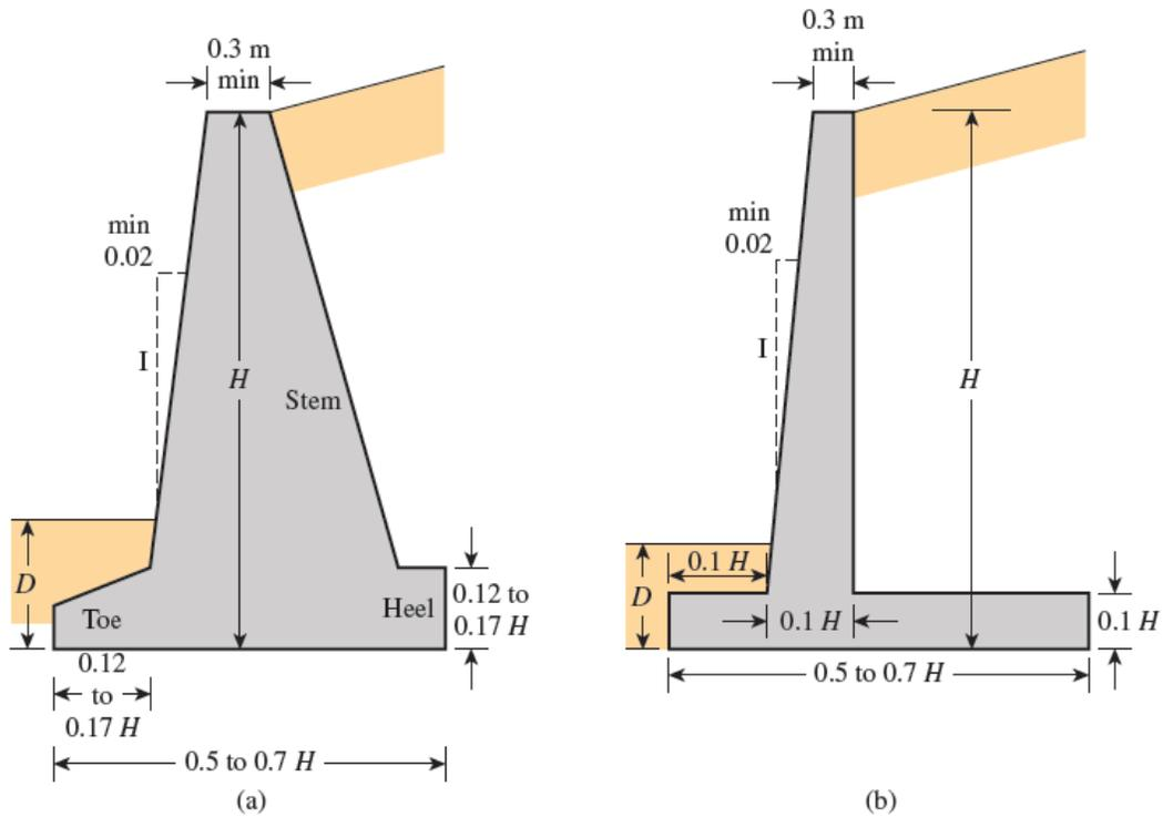
Fig. 11.3 Approximate dimensions for various components of retaining walls for initial stability checks: (a) gravity wall; (b) cantilever wall
