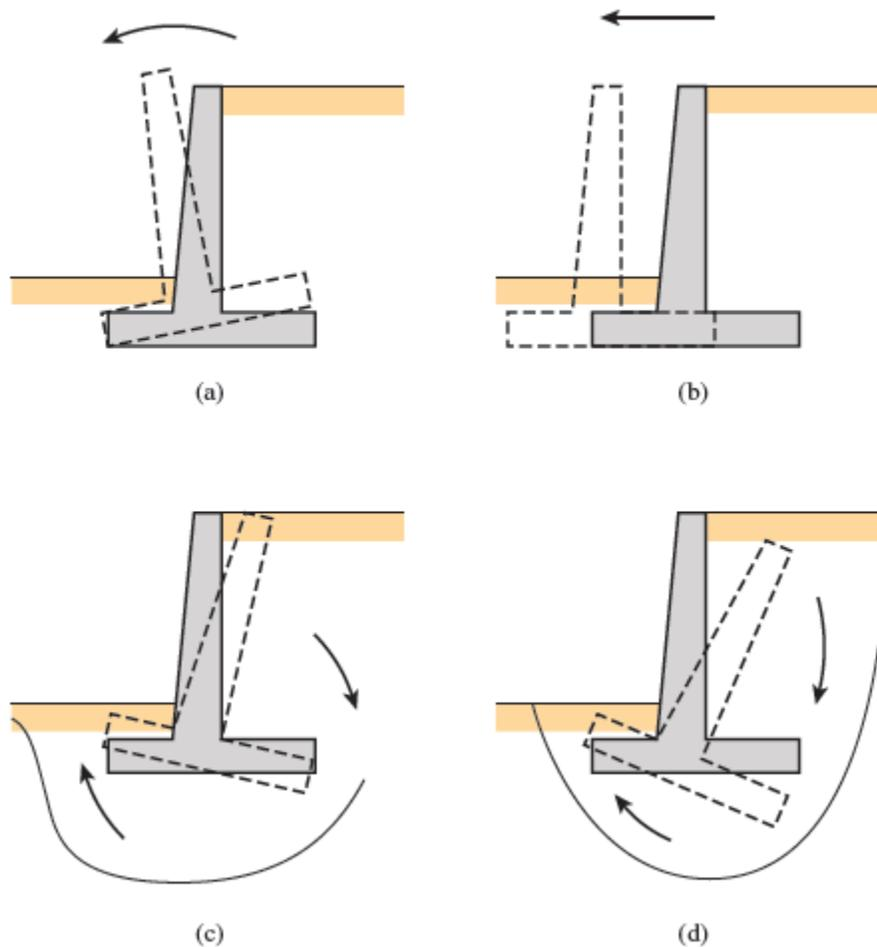
**Fig. 11.4** Failure of retaining wall: (a) by overturning; (b) by sliding; (c) by bearing capacity failure; (d) by deep-seated shear failure
