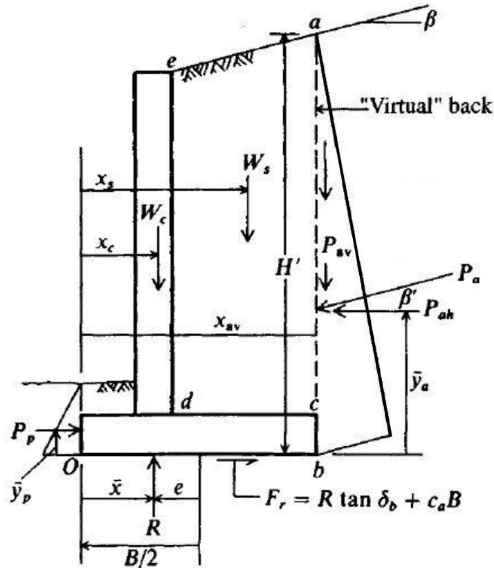
**Fig. 11.5** Wall pressure for overall stability against overturning and sliding.  $W_c$  = weight of all concrete (stem and base);  $W_s$  = weight of soil in zone  $acde$ . Find moment arms  $x_i$  any way practical – usually using parts of known geometry. Use this lateral pressure for base design and bearing capacity.
