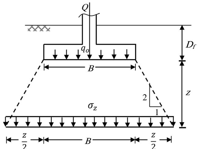
**Fig. 4.3** Stress distribution according to 2:1 slope method
