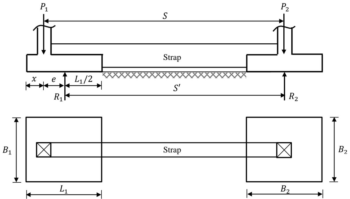
Fig. 6.6 Assumed loading and geometry of strap footing
