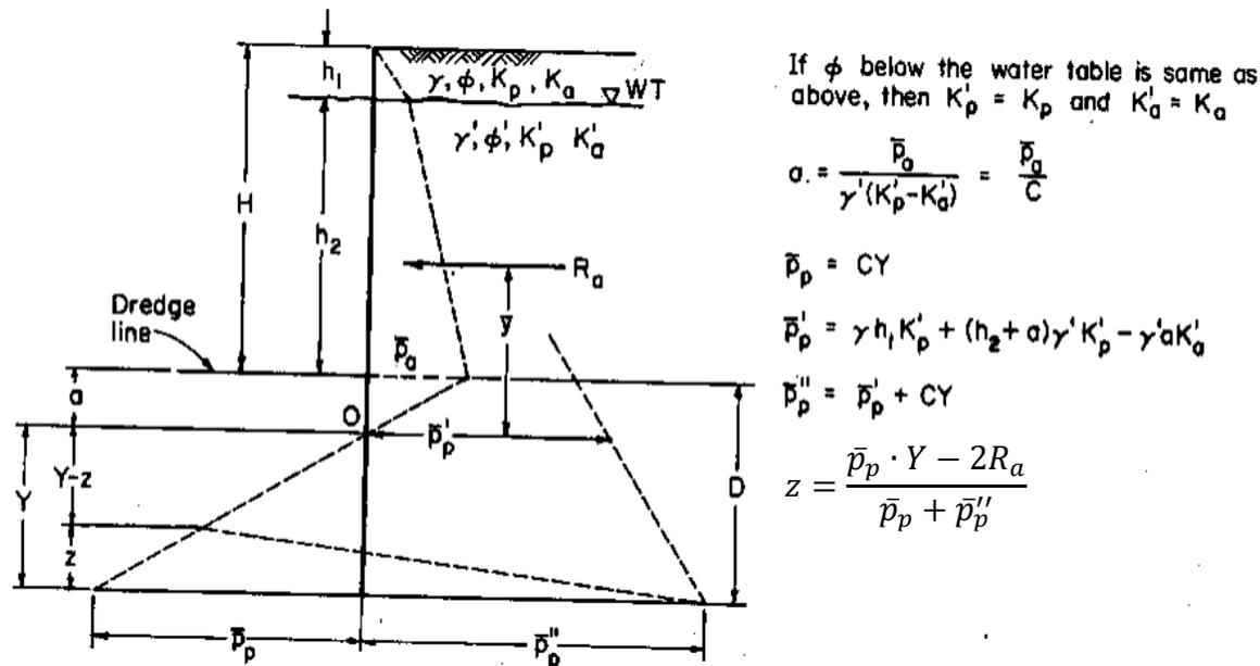
**Fig. 12.3** Cantilever sheetpiling pressure diagram for a granular soil. The diagram illustrates the possibility of different soil properties below the water table. If other stratification exists, the pressure diagram should be appropriately modified.
