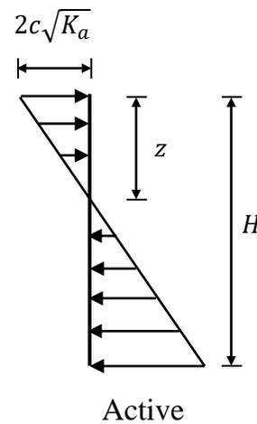
**Fig. 10.4** Active lateral earth pressure distribution for a  $(c - \phi)$  soil
