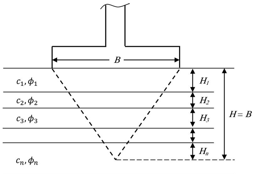
Fig. 3.12 Footing on layered  $c - \phi$  soil
