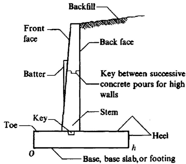
Fig. 11.2 Principal terms used with retaining walls.
