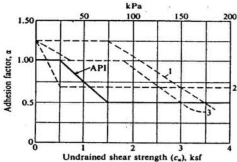
Fig. 8.9  $\alpha - c_u$  relation for different soil conditions
