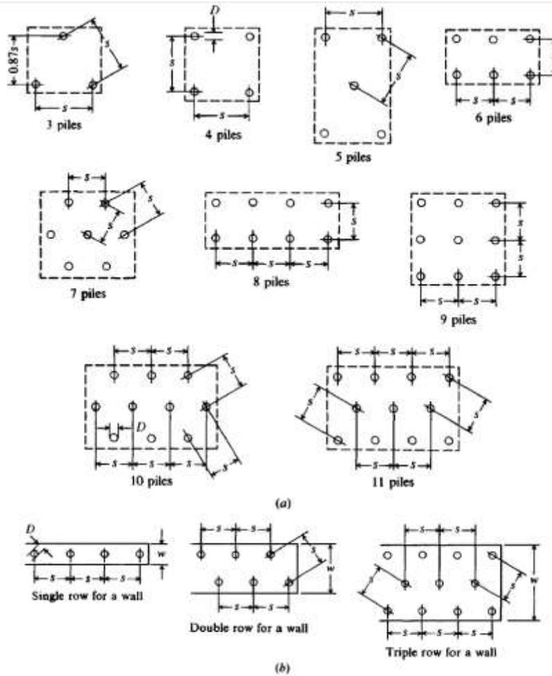
Fig. 9.1 Typical pile-group patterns: (a) for isolated pile caps; (b) for foundation walls.
