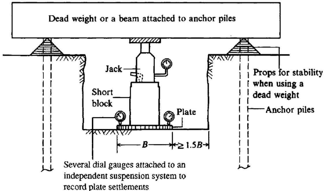
**Fig. 2.19** Plate-load testing. The method of performing this test is outlined in some detail in ASTM D 1194.
