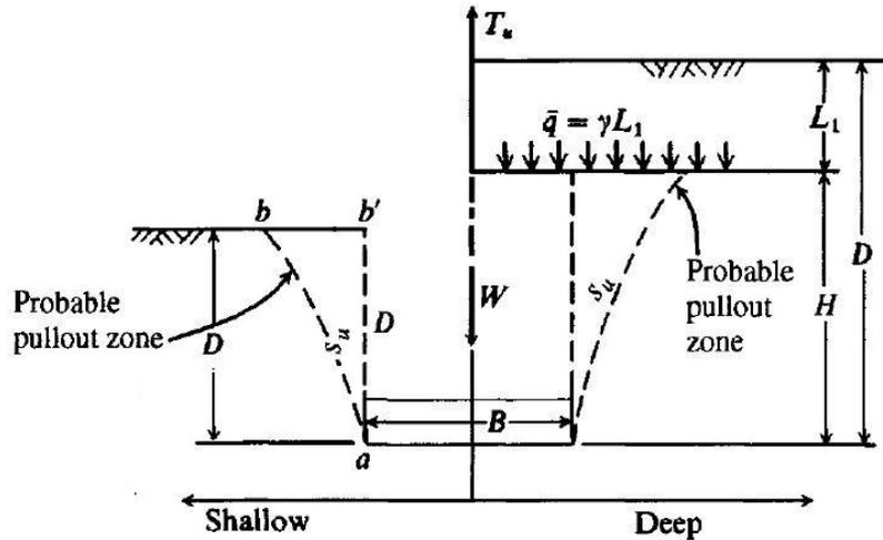
Fig. 3.17 Footings subjected to uplift or tension forces
