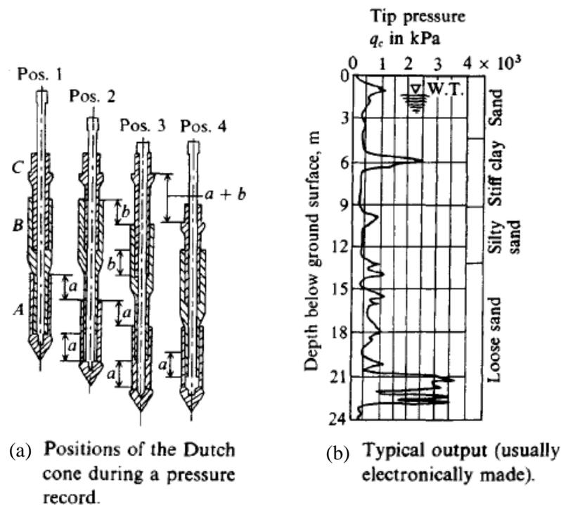
**Fig. 2.16** Mechanical (or Dutch) cone, operations sequence, and tip resistance data
