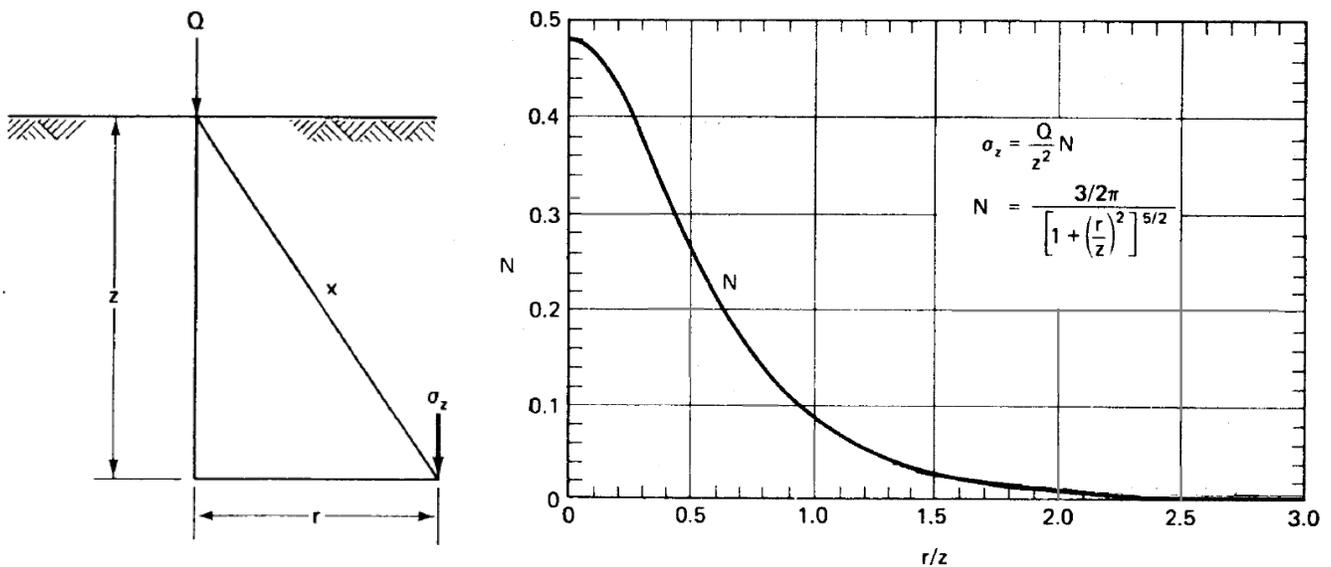
**Fig. 4.4** Vertical stress under point load
