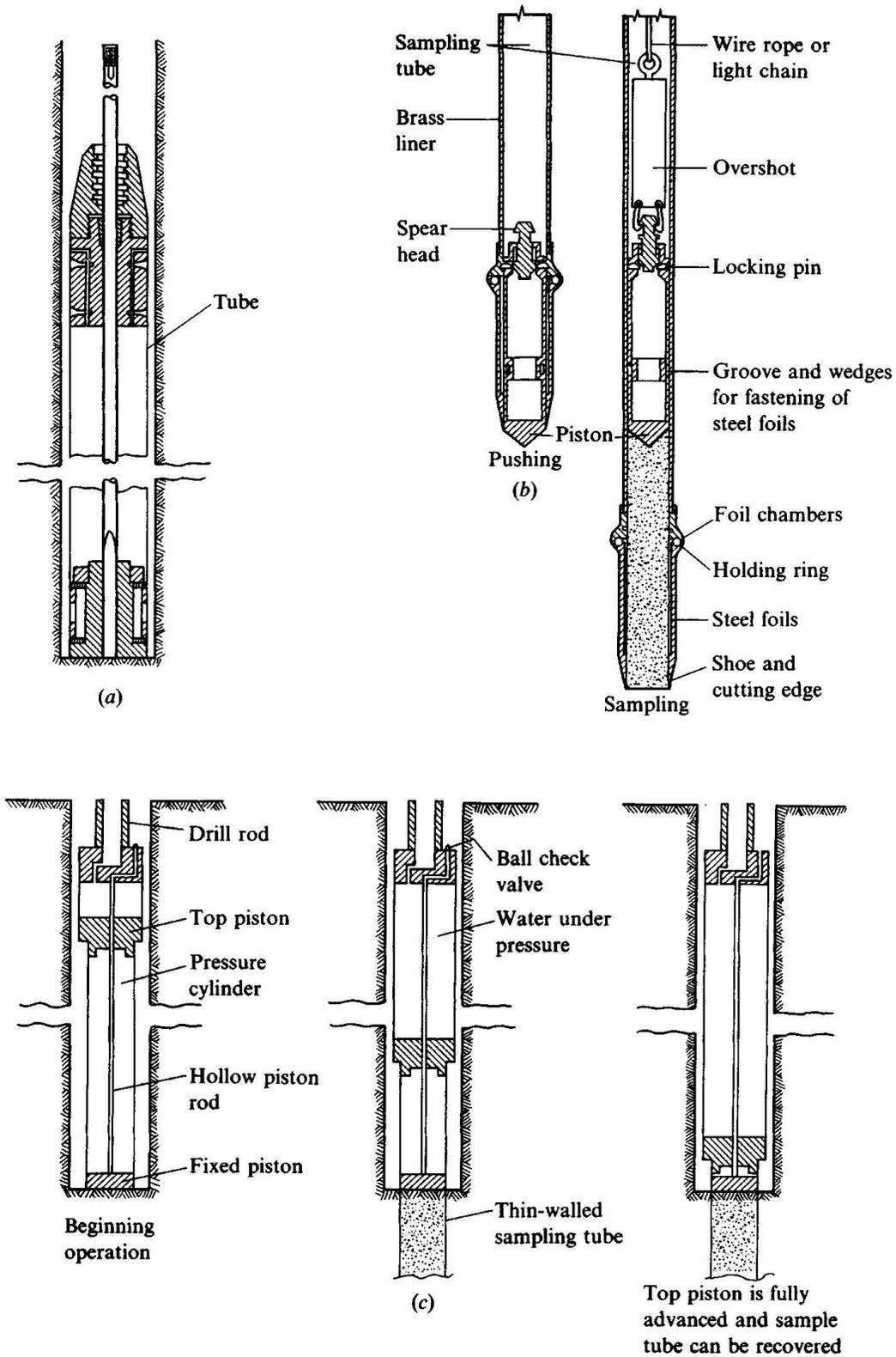
**Fig. 2.8** Typical piston samplers, (a) Stationary piston sampler for recovery of “undisturbed” samples of cohesive soils. Piston remains stationary on soil and tube is pushed into the soil; piston is then clamped and sample is recovered; (b) Swedish foil sampler; (c) Osterberg piston sampler. [Hvorslev (1949)].
