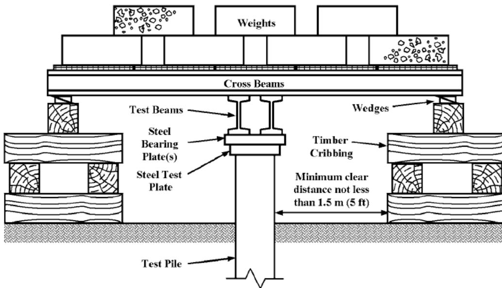
Fig. 8.12 Schematic of direct loading on a single pile using weighted platform
