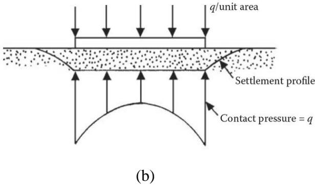
**Fig. 4.1** Flexible (a) and rigid (b) foundations on clay
