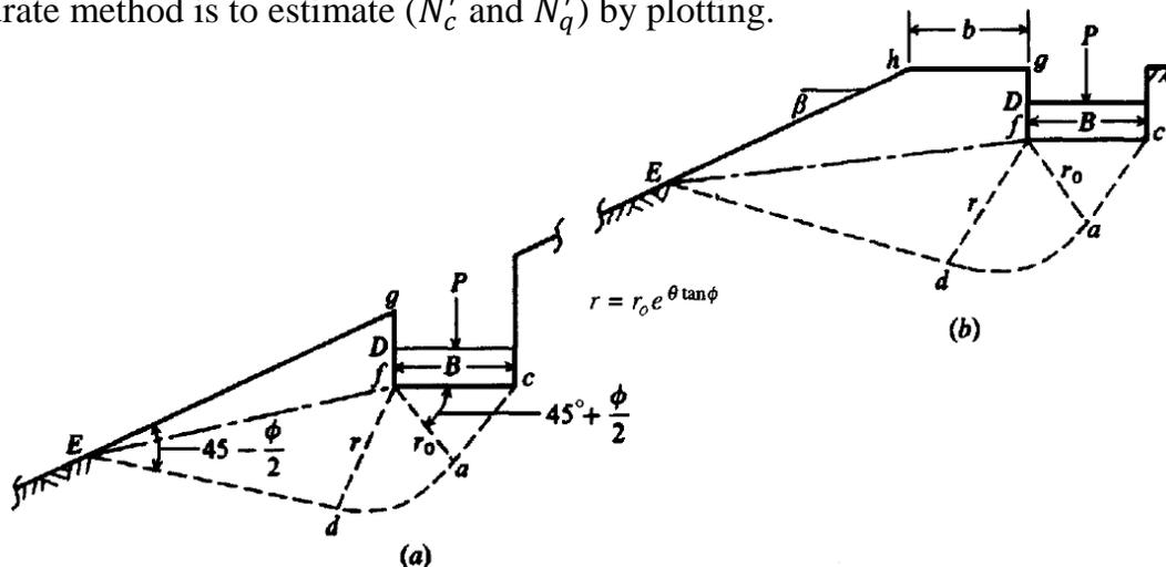
Fig. 3.13 Footings on or adjacent to a slope.
