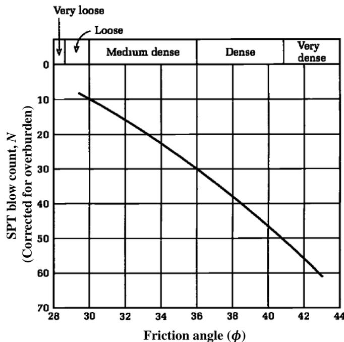
**Fig. 2.15 SPT blow count ( $N$ ) versus friction angle ( $\phi$ )**
