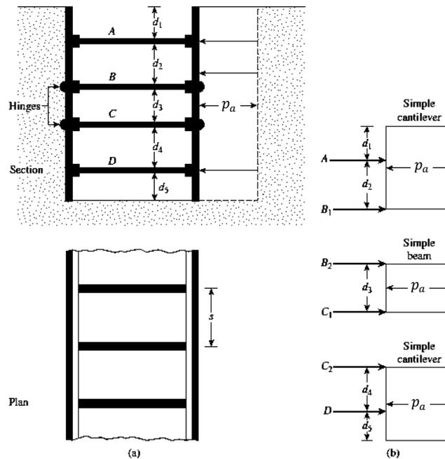
**Fig. 12.10** Determination of strut loads: (a) section and plan of the cut; (b) method for determining strut loads
