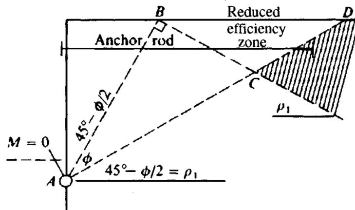
**Fig. 12.7** Locating anchor so active and passive zones do not intersect gives maximum efficiency.
