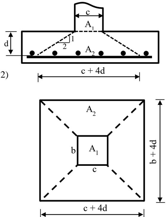
Fig. 5.4  $A_1$  and  $A_2$  for allowable bearing stress
