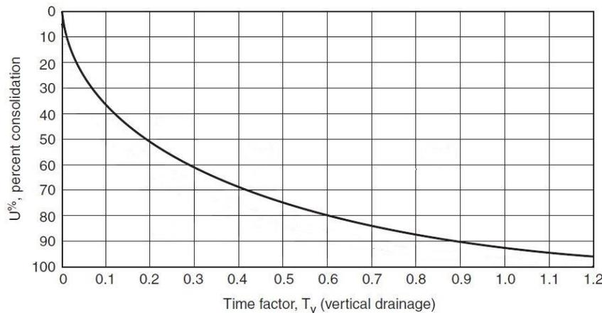
Results of Terzaghi for a linear distribution of excess pore pressure
