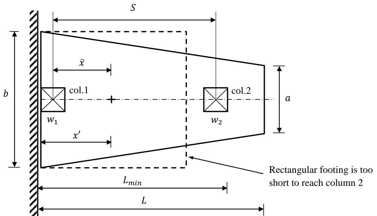
Fig. 6.5 Geometry of trapezoidal combined footing
