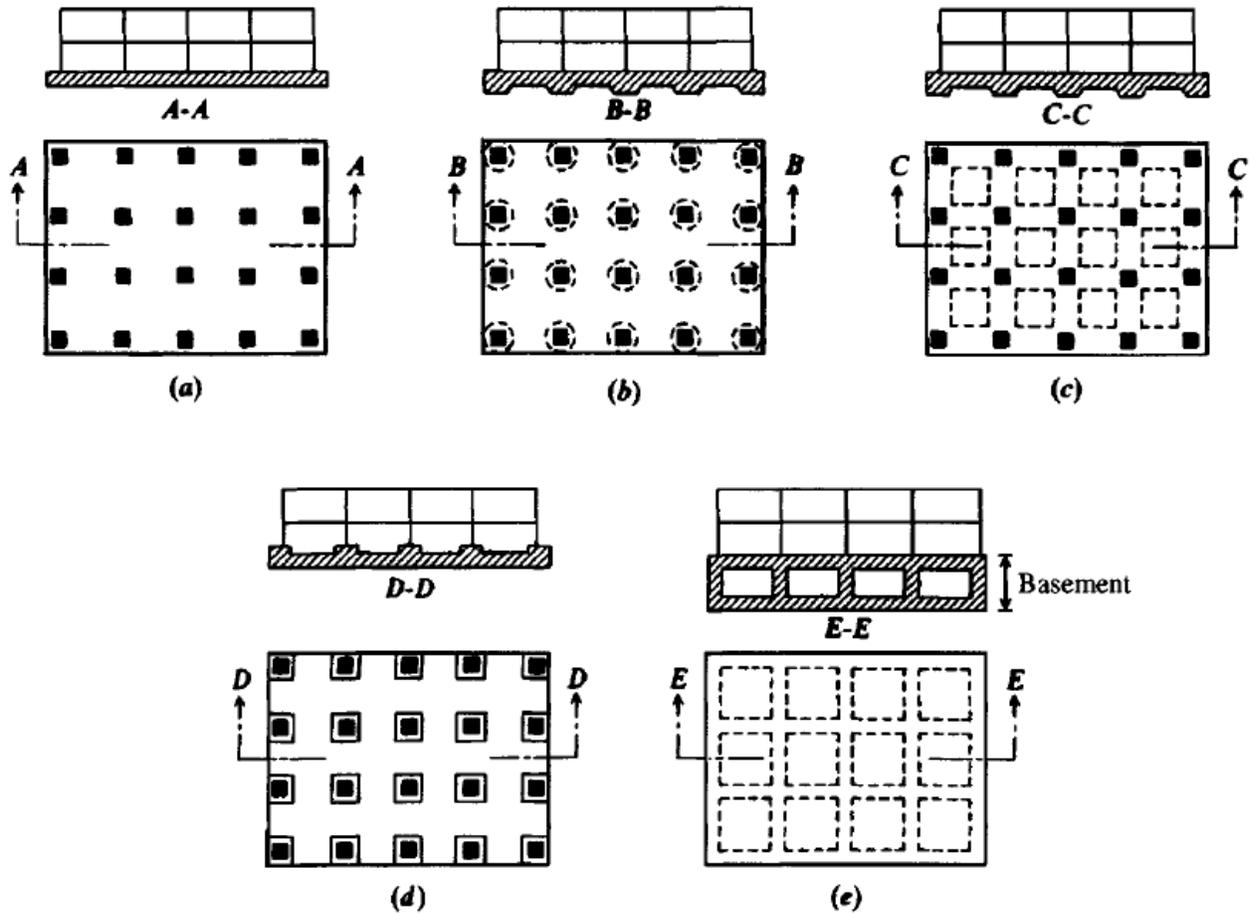
Fig. 7.1 Common types of mat foundations; (a) flat plate; (b) plate thickened under columns; (c) beam-and-slab (waffle slab); (d) plate with pedestals; (e) basement walls as part of mat
