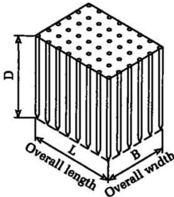
Fig. 9.3 Pile group acting as a block foundation.
