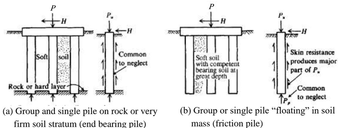
Fig. 8.1 Types of piles based on their resistance
