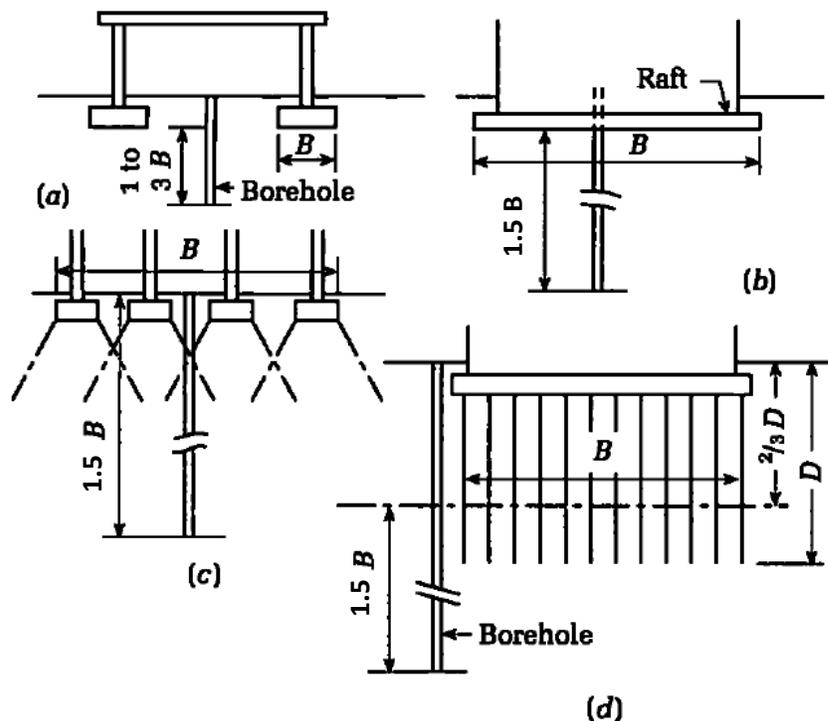
**Fig. 2.11** Depths of boreholes for various foundation conditions
