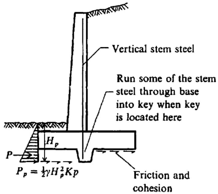
Fig. 11.6 Stability against sliding by using a base key
