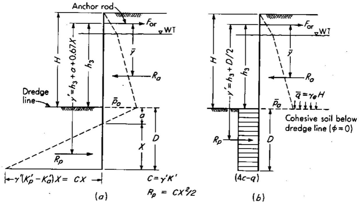
Fig. 12.5 Anchored sheetpiling, free-earth method. (a) All granular soil; (b) cohesive soil below dredge line with granular-soil backfill
