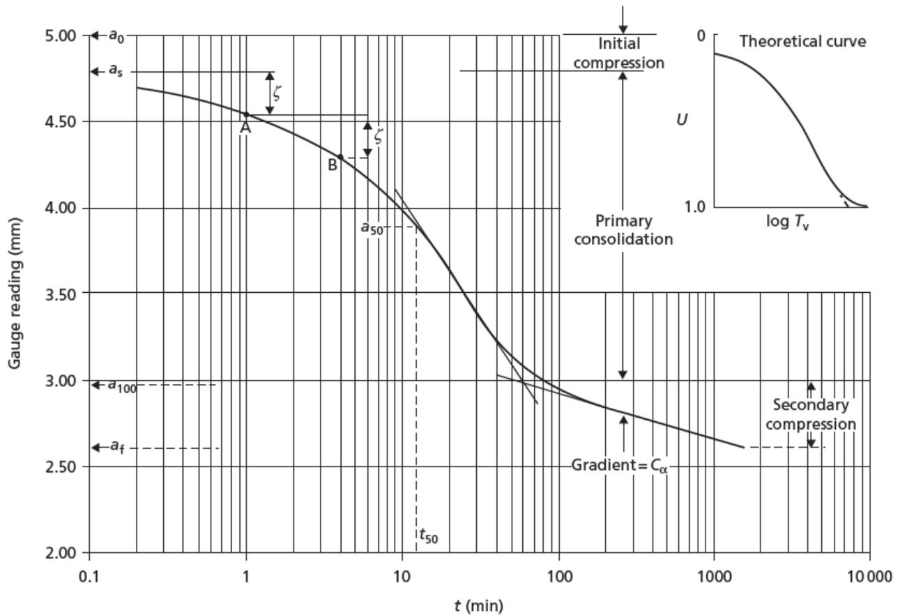
Fig. 4.25 The log time method
