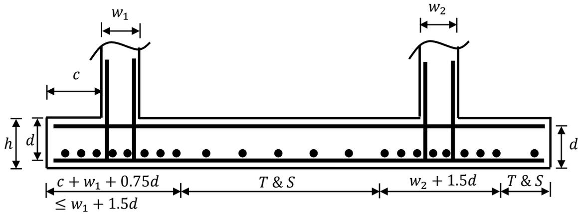
**Fig. 6.4** Details of reinforcement in short direction
