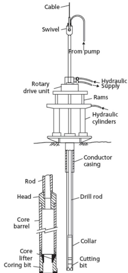
Fig. 2.5 Rotary drilling.
