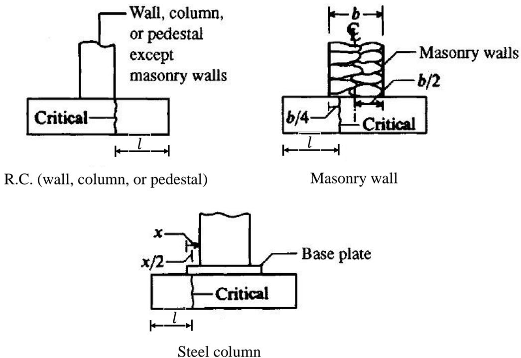
Fig. 5.3 Critical sections for computing bending moment
