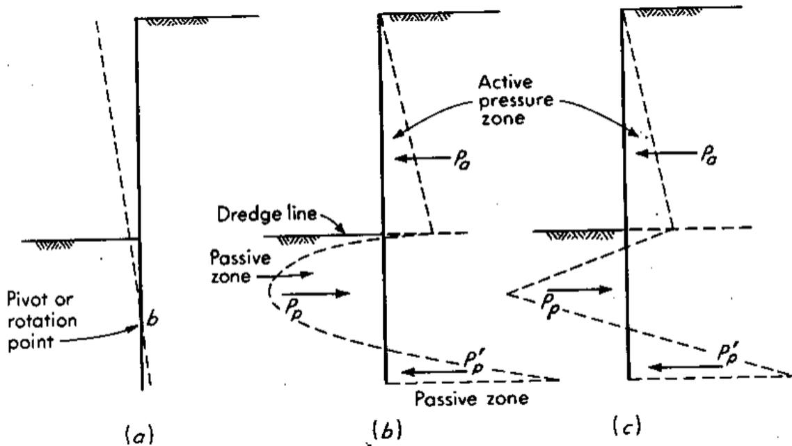
**Fig. 12.2** (a) Assumed elastic line of the sheetpiling; (b) probable and as obtained in finite-element solution qualitative soil-pressure distribution; (c) simplified pressure diagram for computational purposes (granular soil and no water as shown).
