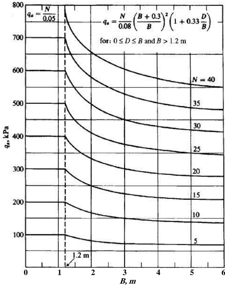
Fig. 3.16 Allowable bearing capacity for surface-loaded footings with settlement limited to approximately 25 mm. Equation used is shown on figure.
