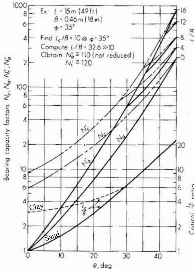
Fig. 8.7 Bearing-capacity factors for deep foundations. [After Meyerhof (1976).]
