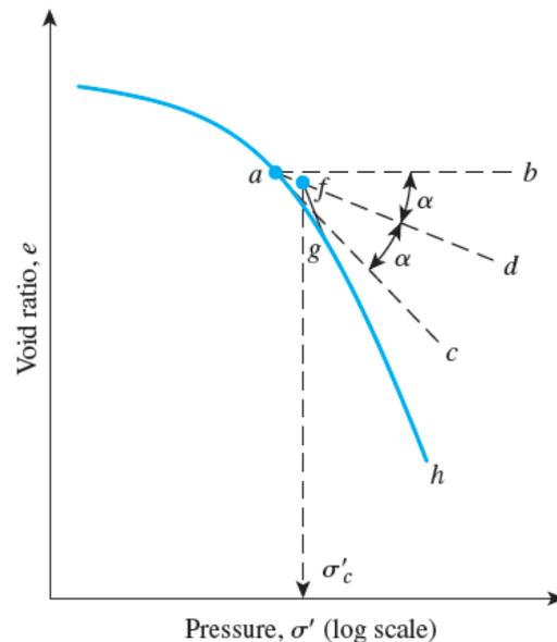
**Fig. 4.15** Graphic procedure for determining preconsolidation pressure
