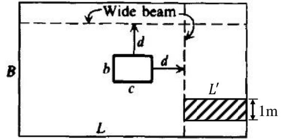
Fig. 5.2 Critical section for wide beam shear
