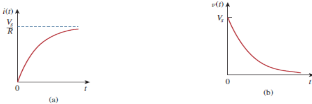
Fig. 2.16 Step responses of an RL circuit with no initial inductor current: (a) current response, (b) voltage response.
