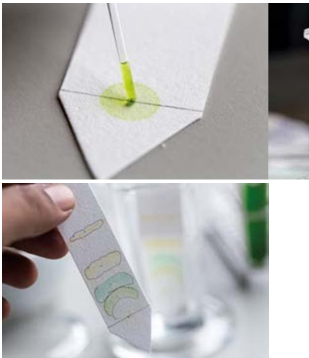
FIGURE 3 Paper chromatography can be used to separate the components of photosynthetic pigment (leaf stain). The pigment is placed on the origin, and then the paper strip is placed in a container where it is in contact with the mobile phase, which is drawn up the paper by capillary action.
