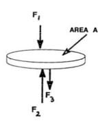
Free-body diagram for the vertical forces acting on an element of fluid at depth D in a hole of cross-sectional area A.
