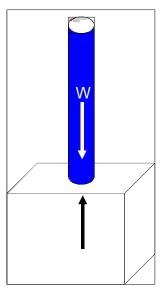
Pressure is the weight of the column of fluid above a unit area.
