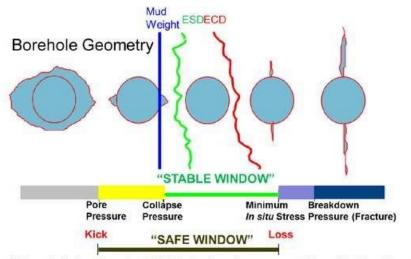
It is important to keep the mud weight higher than the collapse pressure but lower than the minimum in situ stress to maintain hole stability.
