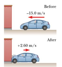
$$\begin{split} p_i &= mv_i = (1.50 \times 10^3 \,\text{kg})(-15.0 \,\text{m/s}) \\ &= -2.25 \times 10^4 \,\text{kg} \cdot \text{m/s} \\ p_f &= mv_f = (1.50 \times 10^3 \,\text{kg})(+2.60 \,\text{m/s}) \\ &= +0.390 \times 10^4 \,\text{kg} \cdot \text{m/s} \\ I &= p_f - p_i \\ &= +0.390 \times 10^4 \,\text{kg} \cdot \text{m/s} - (-2.25 \times 10^4 \,\text{kg} \cdot \text{m/s}) \\ I &= 2.64 \times 10^4 \,\text{kg} \cdot \text{m/s} \end{split}$$
