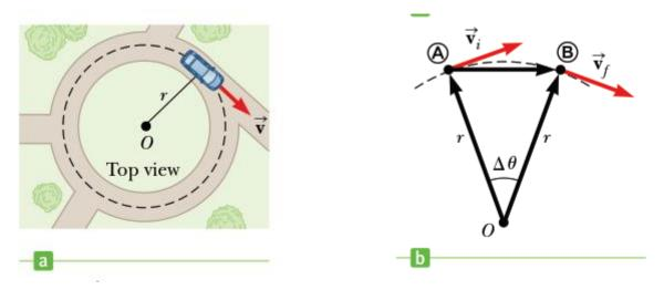
Above Fig. a shows a car moving in a circular path with *constant linear speed* v. Even though the car moves at a constant speed, it still has acceleration. To understand this, consider the defining equation for average acceleration:
