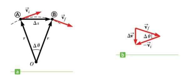
For circular motion at constant speed, the acceleration vector always points toward the center of the circle. Such acceleration is called a *centripetal acceleration* (المركزي المركزي). Its magnitude is given by
