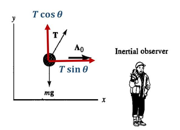
The pendulum hangs at angle  $\theta$  because the railroad car is accelerating in the horizontal direction
