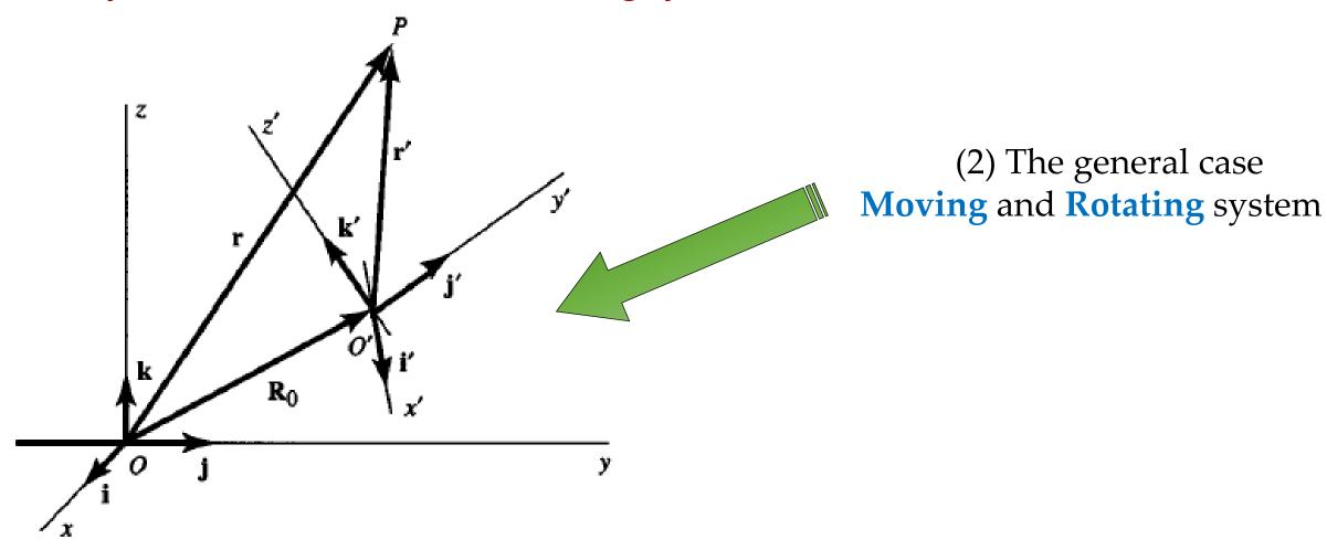
$$v = v' + \omega \times r' + V_0$$
