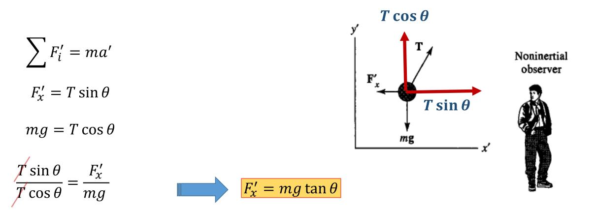
All the forces acting on the pendulum are in balance and the pendulum hangs left the vertical due to the force  $(F'_{\chi} = mg \tan \theta = -mA_0)$
