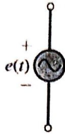
FIGURE( 1-3) Symbol for a sinusoidal voltage source. Lowercase letter e is used to indicate that the voltage varies with time.
