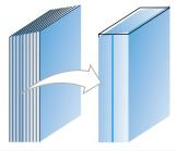
In a thin slab, the cross sections do not vary much in size and shape.
