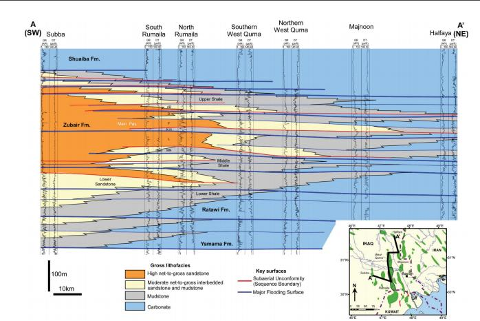
**Figure 4.** Subregional cross section through the Ratawi, Zubair, and Shuaiba formations illustrating the southwest-to-northeast pinch-out of successive Zubair sandstone tongues and the overall regressive—transgressive nature of the Zubair Formation. Key surfaces are tentatively correlated in the authors' absence of biostratigraphic data outside of Rumaila.
