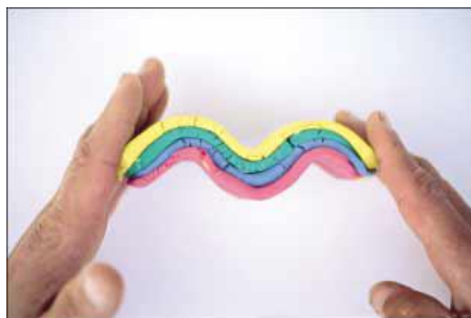
Figure 1-8 Clay deforms into a sequence of folds when compressed
