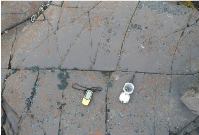
Fig. 1-35 Note how the rock is broken into rectangular blocks, a common phenomenon when two orthogonal (at right angles) joint sets exist. Also note how the one set of joints truncates against the continuous joint running from side to side in the image. If this relationship is consistent, the continuous joint is the longitudinal joint, which is interpreted to have formed before the cross joints that truncate against it. Finally note that some fractures that can not be assigned to one of the two orthogonal sets exist. It is not uncommon at all that a rock body can have three or more joint sets developed within it.
