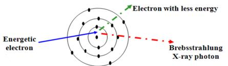
As the electrons pass through the target atom they slow down, with a loss in kinetic energy. This energy is emitted as x-rays.
