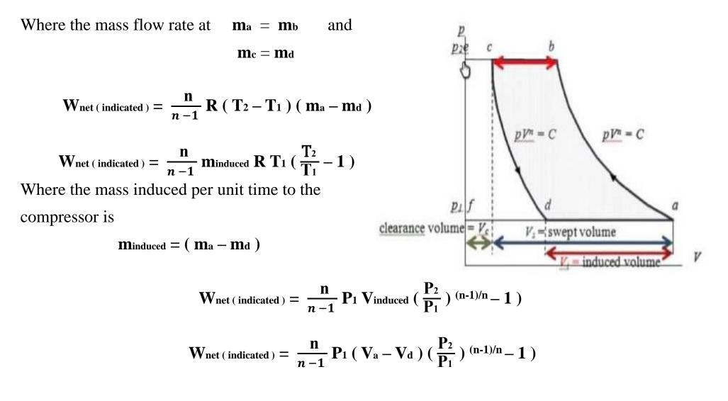
Where the volume induced per unit to the compressor is  $V_{induced} = (V_a - V_d)$
