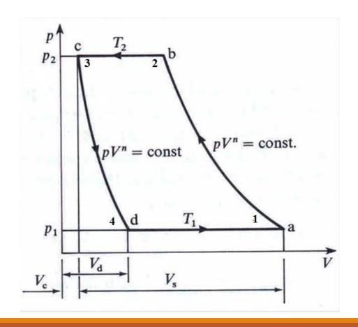
Process da is isobaric expansion, the perfect gas ( air ) expand according to the law of work :
