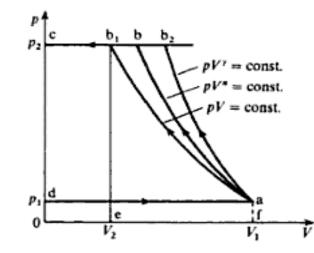
compressor the gas temperature must be kept as close as possible to its initial value, and a means of cooling the gas is always provided, either by air or by water.
