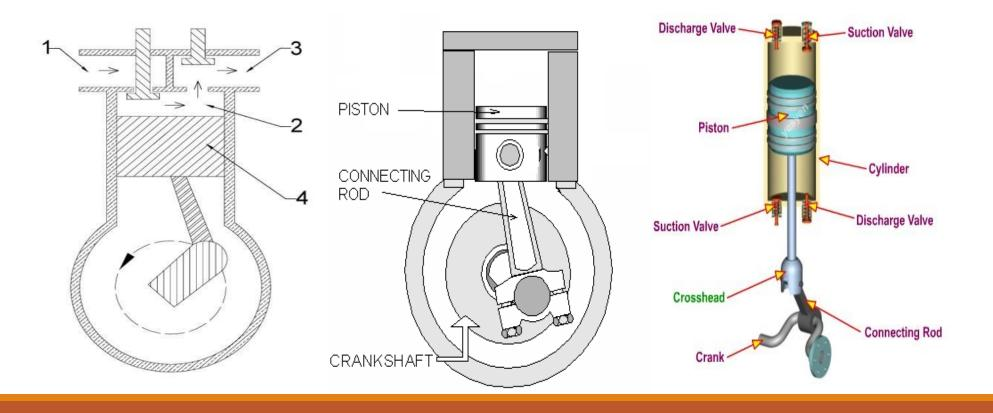
Reciprocating compressors are positive displacement machines in which the compressing and displacing element is a piston having a reciprocating motion within a cylinder.
