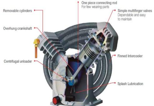
The **Thermodynamic Cycle**. An explanation of a few basic **thermodynamic** principles is necessary to understand the science of **reciprocating compressors**. Compression occurs within the cylinder as a four-part **cycle** that occurs with each advance and retreat of the piston (two strokes per **cycle**).
