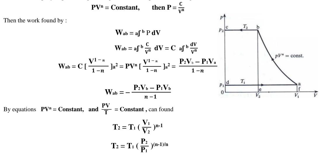
Process ab is isobaric, the perfect gas (air) compress according to the law of work :
