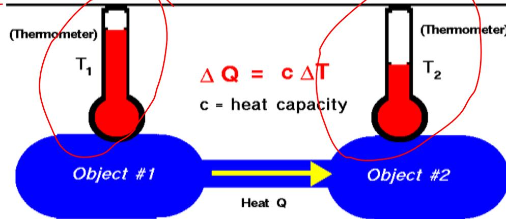
In the process of reaching thermodynamic equilibrium, heat is transferred from the warmer object to the cooler object. At thermodynamic equilibrium heat transfer is zero.
