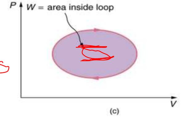
The negative area below path CD subtracts, leaving only the area inside the rectangle. In fact, the work done in any cyclical process (one that returns to its starting point) is the area inside the loop it forms on a  $PV$  diagram, as Figure (c) illustrates for a general cyclical process. Note that the loop must be traversed in the clockwise direction for work to be positive—that is, for there to be a net work output.
