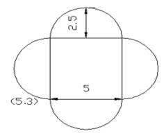
**Example (3-3)** Draw the following figure. Note the figure is start from original point (0, 0).
