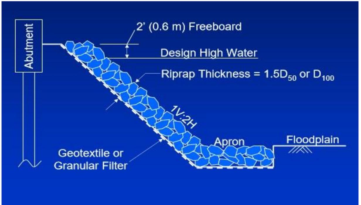
Fig 2 : Cross section of Abutment Riprap
