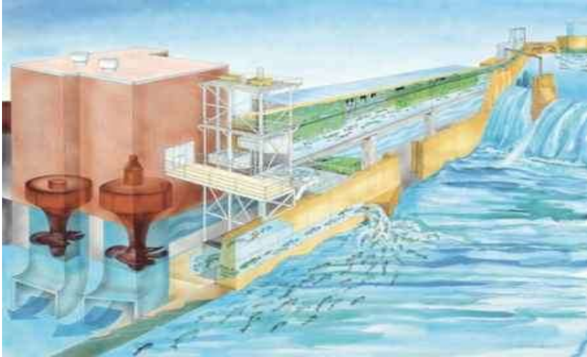
Fig (8-40) Fish Lifting Procedure, Holyoke Dam, USA
