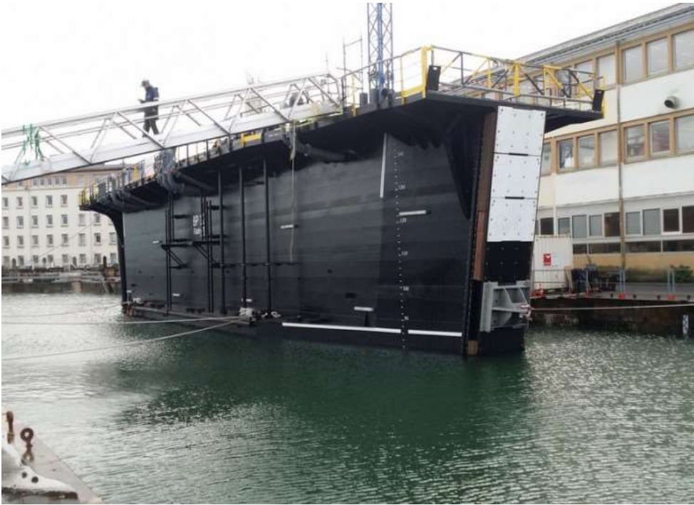
Fig (6.8) Side Floating Dry Dock
