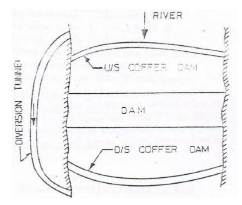
Figure 1.2 Main dam with coffer dam and diversion tunnel
