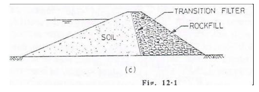
Figure (2.1) (a) Earth dam. (b) Rockfill dam. (c) Composite Earth And Rockfill Dam
