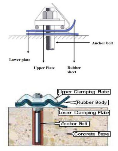
Figure (6.7) Steel Clamps with Anchor Bolts
