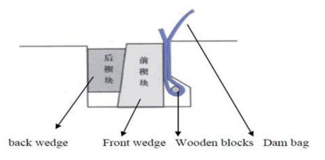
Figure (6.6) Concrete Wedge Blocks
