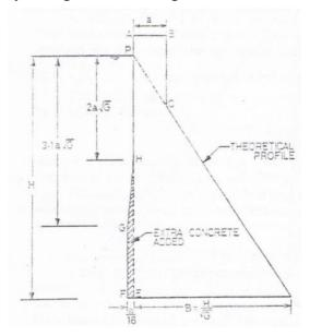
Figure (3.20) practically profile of a gravity dam.
