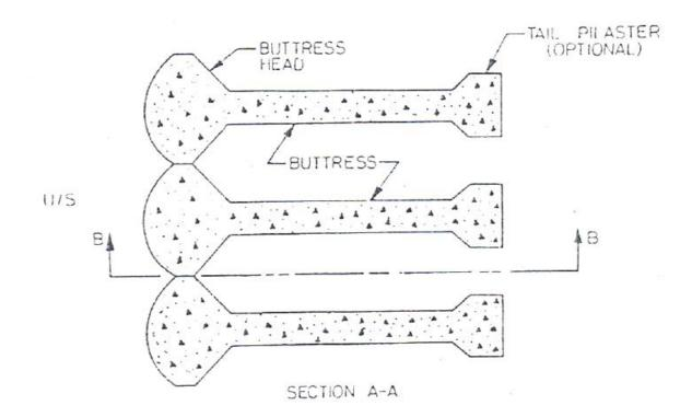
Figure (5.3) massive head buttress dam.
