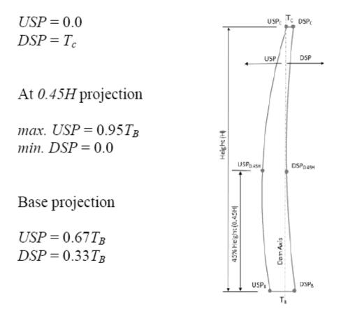
Figure (4.5) double curvature arch dam
