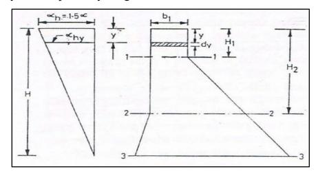
Figure (3.13) Seismic coefficient method.
