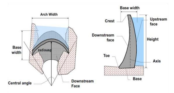
Figure (4.3) cross section of arch dam
