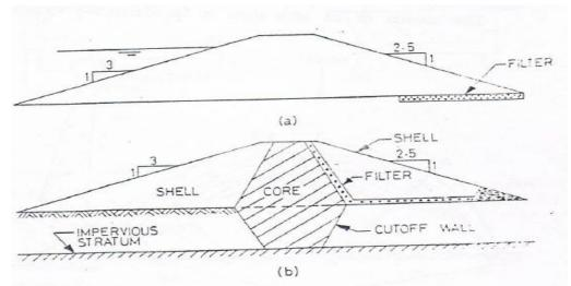
Figure 1.7 Earth dam component
