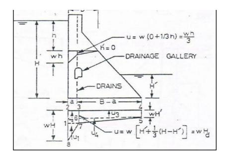
Figure (3.10) Effect of drains on uplift pressure.
