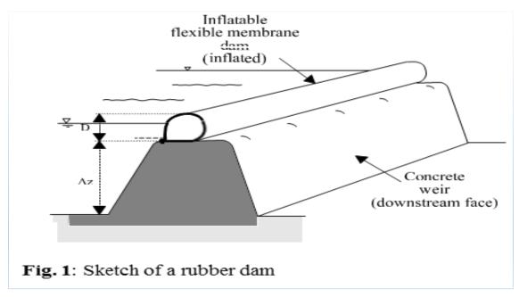
Figure (6.1) Sketch of a rubber dam
