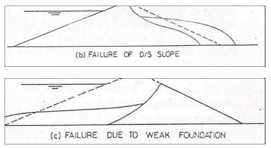
Figure (2.9) (a) Failure of U/s slope during sudden drawdown. (b) Failure of D/s slope during steady seepage.(d) Failure due to weak foundation.
