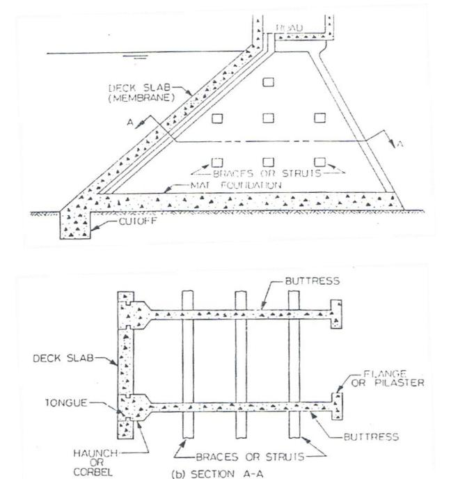
Figure (5.1) deck slab buttress dam.
