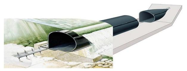
Figure (6.5) components of Rubber dam
