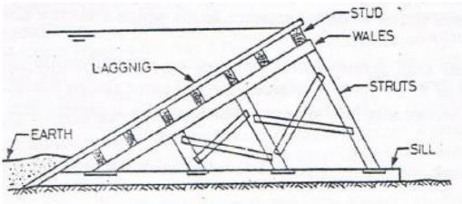
Figure 1.13 A frame timber dam
