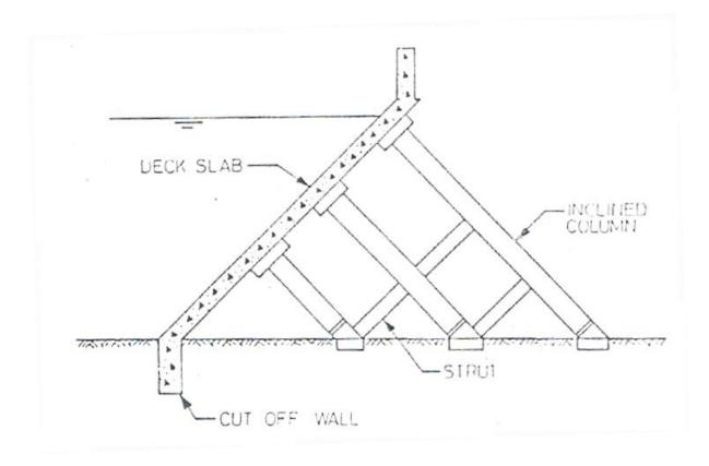
Figure (5.4) columnar buttress dam.
