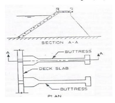
Figure 1.10 Deck type buttress dam
