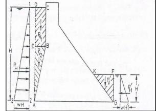
Figure (3.5) gravity dam with U/s inclined face.
