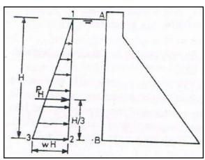
Figure (3.4) gravity dam with U/s Vertical face.
