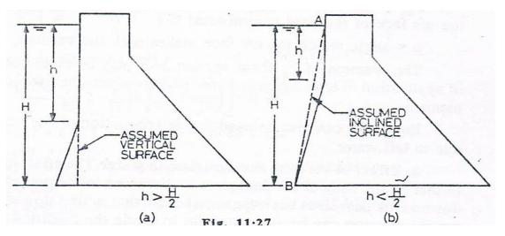
Figure (3.23 a and b) partly vertical and partly sloping U/S face dam.
