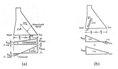
Figure (3.16) vertical stress distribution for (a) reservoir full case, (b) reservoir empty case.
