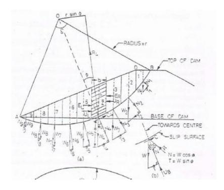
Figure 2.10 the stability of slopes of the earth dam.
