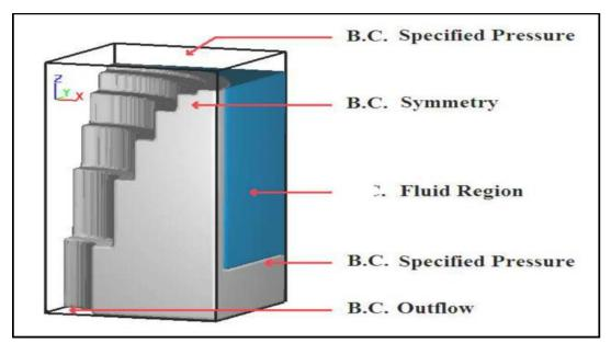
Figure 4: Boundary and initial conditions for SMGS model.
