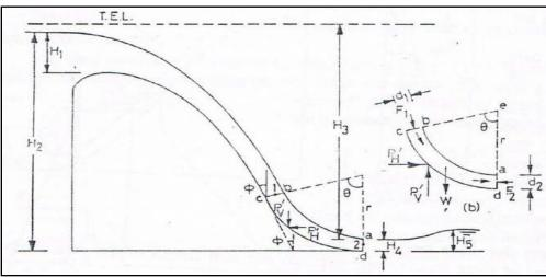
Figure (3.8) gravity dam Dynamic pressure on the D/s face.
