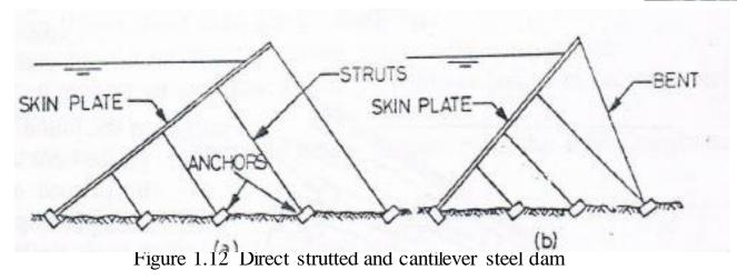
Note: The steel dam quite costly and subjected to corrosion. These dam are almost obsolete. Steel dams are sometimes used as temporary coffer dam.
