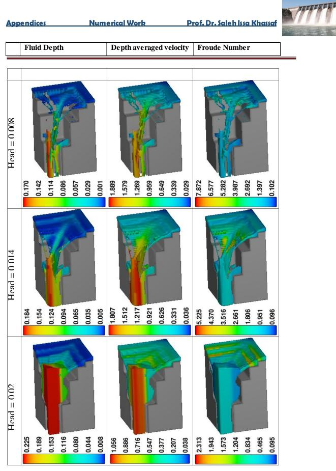
Figure 7: Four steps quadrate SMGS model results of FLOW 3D simulation.
