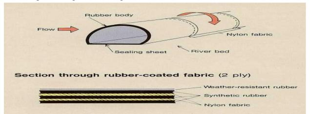
Figure (6.3) Materials of Rubber dam
