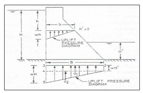
Figure (3.9) Total uplift force on the base of the dam.
