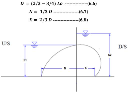
Figure (6.4) Shape of Rubber dam
