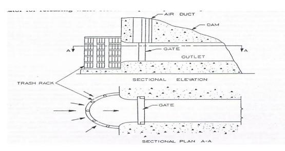
Figure (8.1): Section of outlet.
