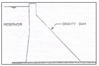
Figure (3.1) Gravity dam.
