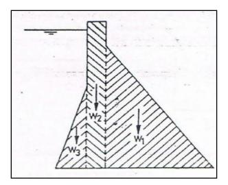
Figure (3.3) Computation The weight of the dam.
