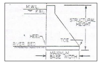
Figure (3.2) Basic Definitions of gravity dam.
