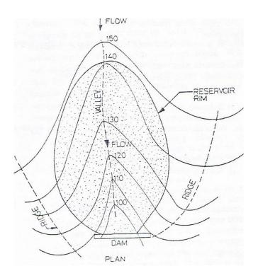
Figure (7.1) Plan of Reservoir
