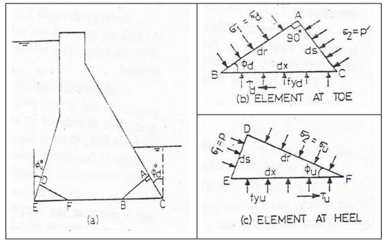
Figure (3.17) principal stress acting in a gravity dam.
