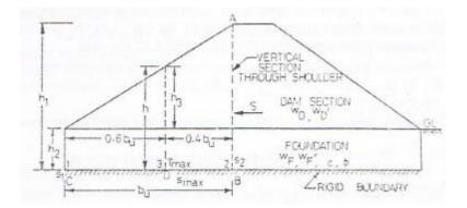
Figure 2.14 shows the upstream portion of an earth dam on a weak foundation.
