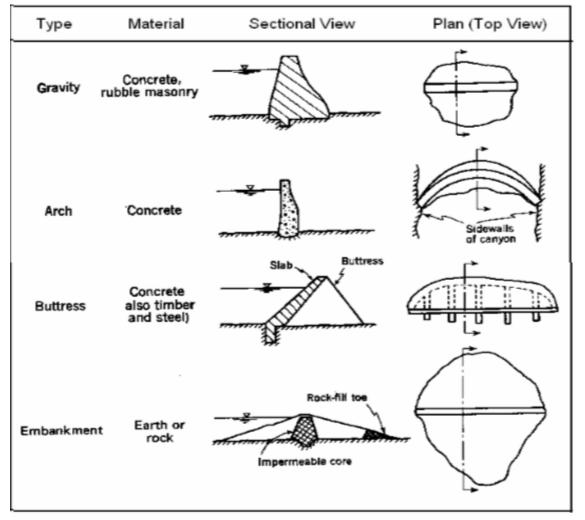
Figure 1.4 Dams type according to material construction
