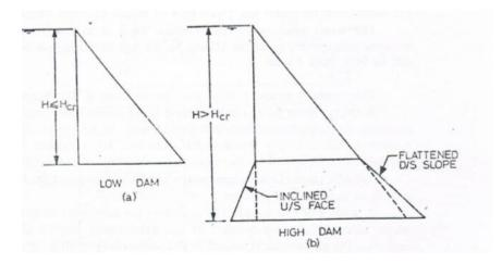
Figure (3.19) distinction of the of low and high gravity dam. (a) low dam, (b) high dam.
