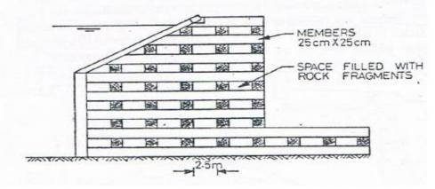
Figure 1.14 Rock-filled crib rock dam
