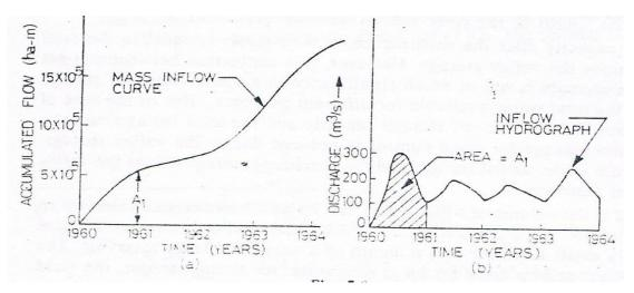
Figure (7.5) M ass Inflow Curve and Hydrograph.
