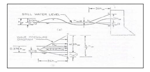
Figure (3.11) Effect Wave Pressure on gravity dam.
