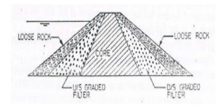
Figure 2.16 shows the cross-section of an earth dam in a seismic zone.
