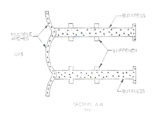
Figure (5.2) multiple arch buttress dam.
