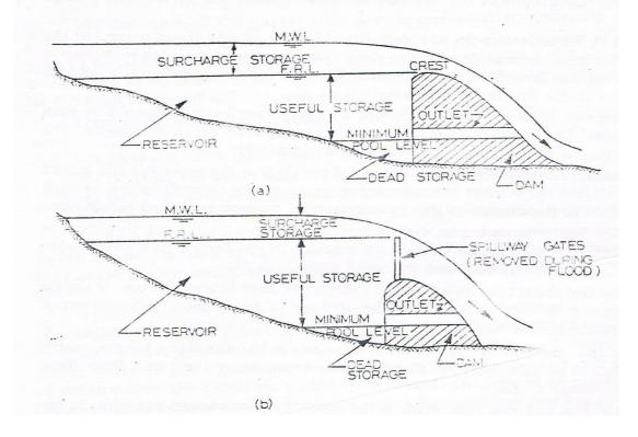
Figure (7.4) Gated and Ungated Spillway
