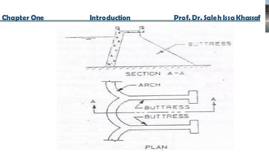
Figure1.11 Multiple-arch type buttress dam
