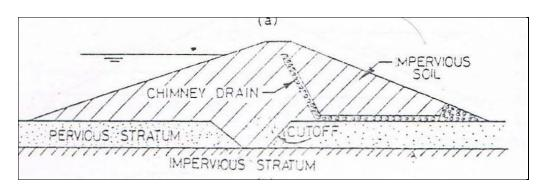
Figure (2.7) The chimney drains as drainage system.
