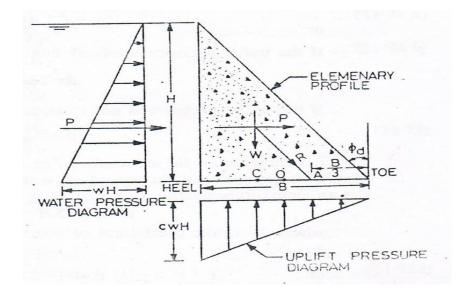
Figure (3.18) elementary profile of gravity dam.
