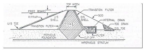
Figure (2.5) Section of Earth Dam.
