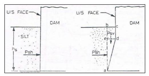
Figure (3.12) Effect silt Pressure on gravity dam.
