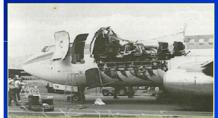
Failed fuselage of the Aloha 737 aircraft in 1988.
