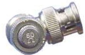
50-ohm resistor on T-connector
