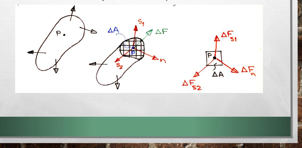
$\Delta F$  is the force acting on an element of area  $\Delta A$ .
