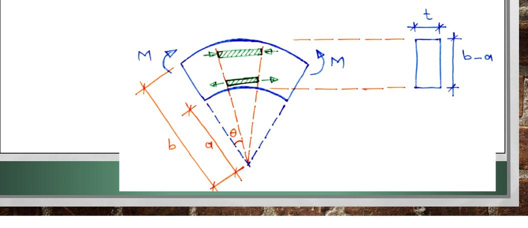
The bending moment constant along the length of the bar and the stress distribution is the same in all radial cross sections.
