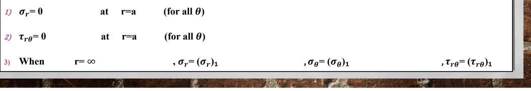
The stresses must be derived from a stress function  $\phi$  which must satisfy the compatibility equation
