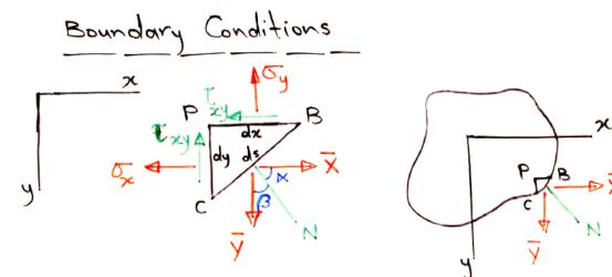
Taking the small triangular prism PBC so that the side BC coincides with the boundary of the body, and denoting by  $\overline{x}$  and  $\overline{y}$  the components of the surface forces by unit area, then
