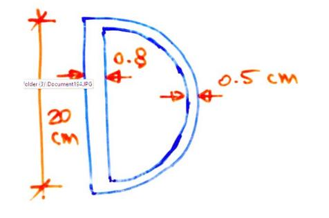
The angle of twist per unit length is
