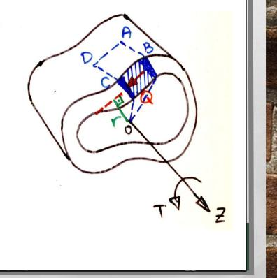
i.e., the product of the shear stress and the thickness is constant at all points on the periphery of the tube. This constant is termed the shear flow and denoted by the symbol q (shear force per unit length ). Thus
