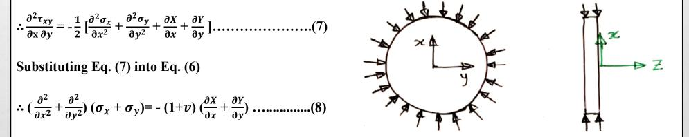
The case of plane stress represents, with only a very small error, the state of stress in a thin plate which is subjected to forces applied at the boundary, parallel to the plane of the plate, and uniformly distributed over the thickness.
