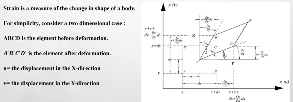
Physically, small displacement means  $A'P \approx A'C'$  and  $\measuredangle PA'C'$  is also small (i.e.,  $\tan \theta \approx \theta$ )
