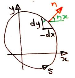
Eq.(7) shows that the stress function  $\psi$  (x,y) must be constant along the boundary of the cross section. The value of  $\psi$  at the boundary can be chosen arbitrarily. It is usually conveniently made equal to zero, i.e.,  $\psi$  (x,y) = 0 on the boundary.
