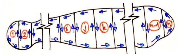
One such equation (Eq.2 or 3) may be written for each of the n cells, and the resulting n linearly independent equations plus the equation
