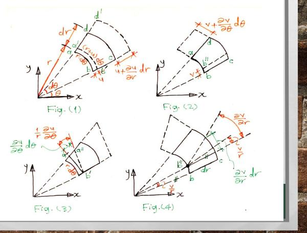
Referring to Fig.(1), a u displacement od side ab results in both radial and tangential strain. The radial strain  $\epsilon_r$  is
