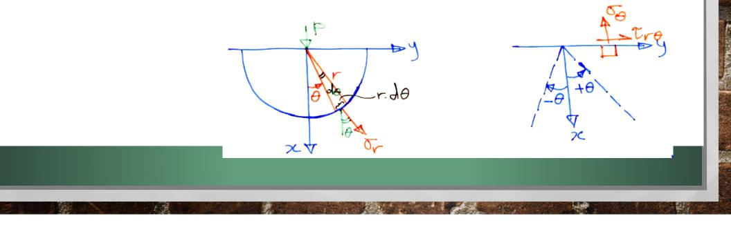
The second of Eqs. (3) can be obtained by considering the vertical equilibrium of semi –circular portion of constant
