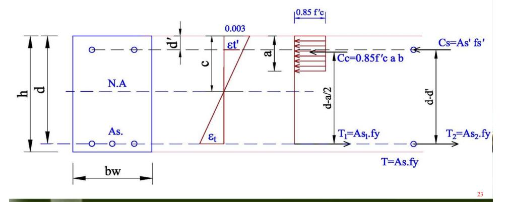
Example (4): A beam section is limited to a width b = 250mm. and a total depth h = 550 mm and has to resist a factored moment of 307 KN.m. Calculate the required reinforcement. Given:  $f'_c = 21$  mPa and  $f_y = 350$  mPa. d' = 65 mm.
