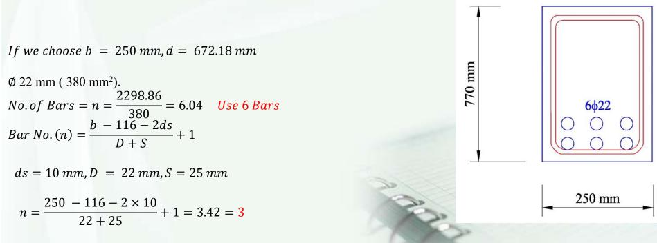
If use two layer h = d + 90 mm = 762.18 mm use h = 770 mm (increase the value for 10 mm)
