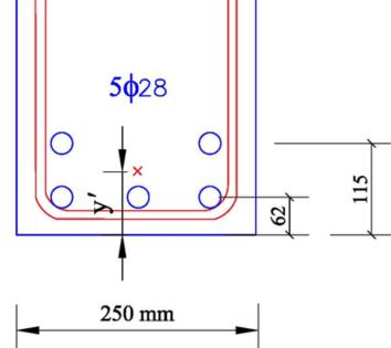
$Max \ As = \frac{(1000 - 250) \times 100}{23.53} + \ 0.01433 \times 250 \times 370 = 4513 \ mm^2 > As = 3075 \ mm^2$   $c = \frac{a}{\beta_1} = \frac{70.68}{0.85} = 83.15 \ mm$   $\epsilon_t = \left(\frac{dt - c}{c}\right) \times 0.003 = \left(\frac{391.5 - 83.15}{83.15}\right) \times 0.003 = 0.0113 > 0.005 \ OK \qquad \emptyset = 0.9 \ T.C$
