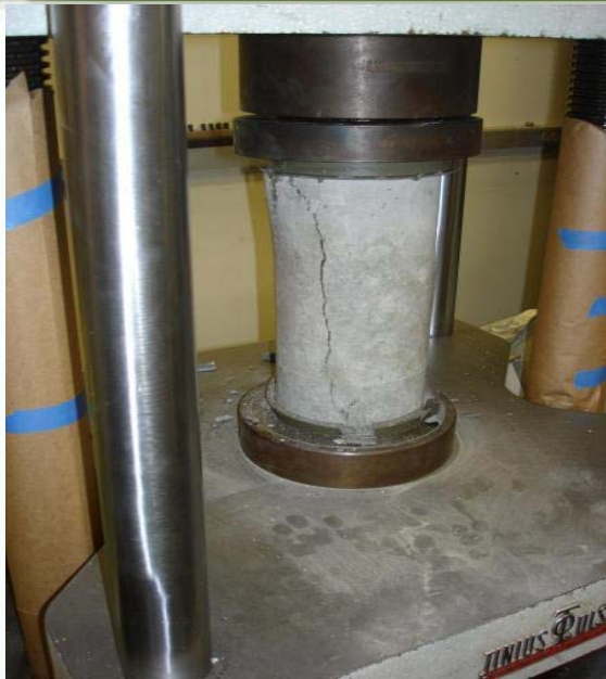
compressive strength test For cylinder
