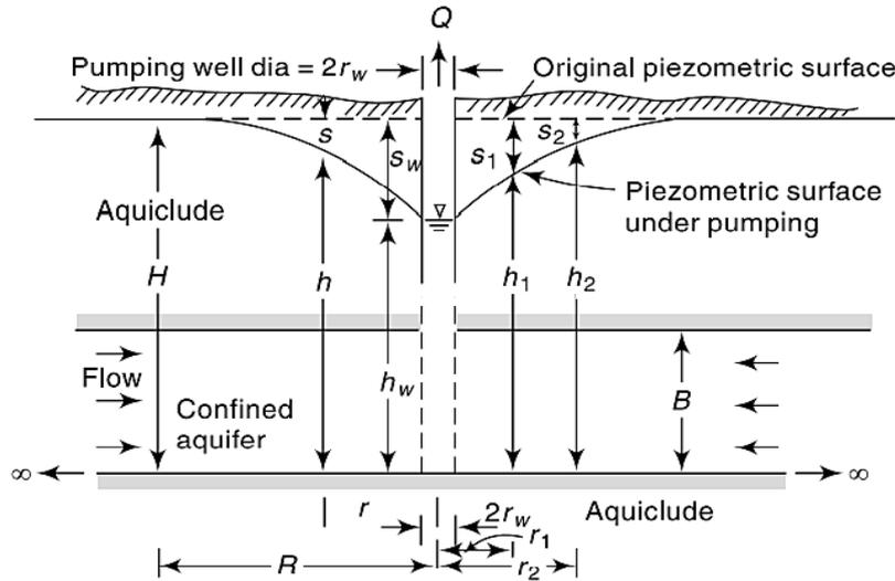
Fig. 2.15 : Well Operating in a Confined Aquifer
