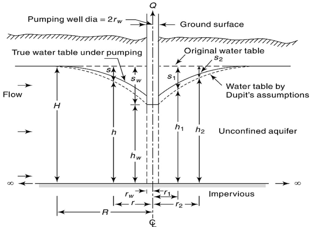
Fig. 2.16 : Radial Flow to a Well in an Unconfined Aquifer
