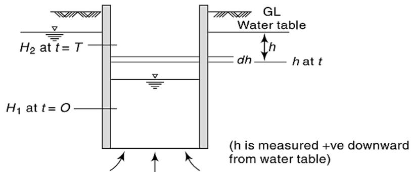
**Fig. 2.17:** Recuperation Test for Open well
