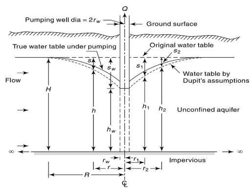
Fig. 2.16: Radial Flow to a Well in an Unconfined Aquifer
