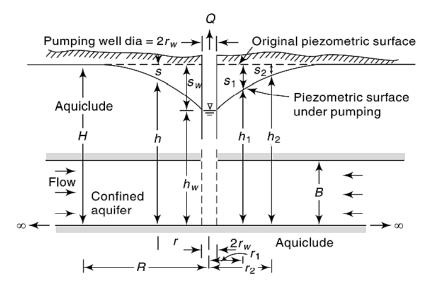
Fig. 2.15: Well Operating in a Confined Aquifer
