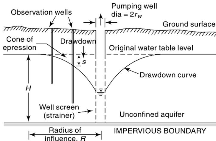
Fig. 2.14 : Well Operating in an Unconfined Aquifer, (definition sketch)
