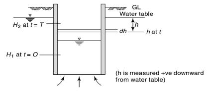
Fig. 2.17: Recuperation Test for Open well
