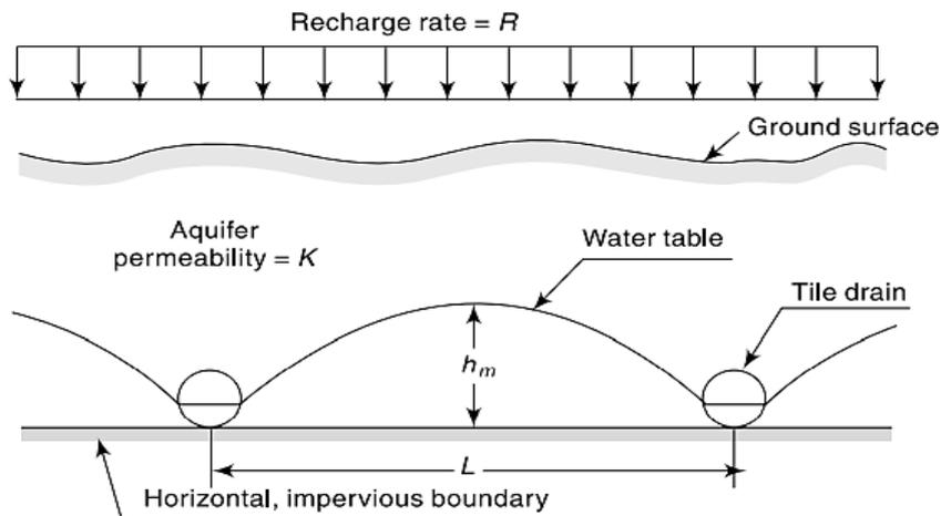
Fig. 2.12: Tile Drains under a Constant Recharge Rate
