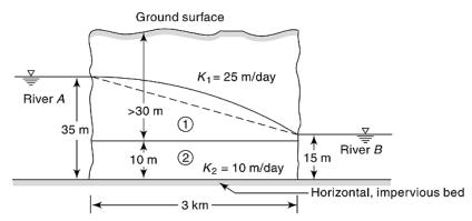
Fig. 2.13: Schematic Layout of Example
