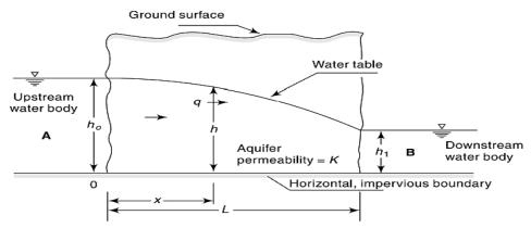
Fig. 2.11: One Dimensional Unconfined Flow without Recharge
