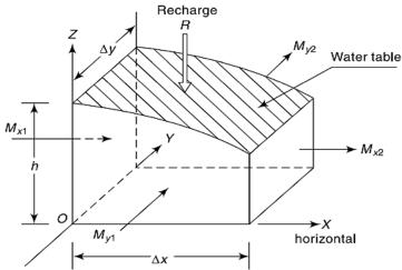
Fig. 2.9 (b): Definition Sketch - Unconfined flow with Recharge
