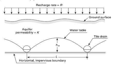
Fig. 2.12: Tile Drains under a Constant Recharge Rate
