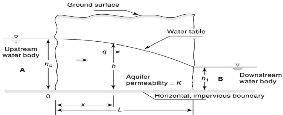
Fig. 2.11: One Dimensional Unconfined Flow without Recharge
