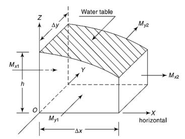
**Fig. 2.9 (a)** :Definition Sketch — Unconfined Groundwater Flow without Recharge
