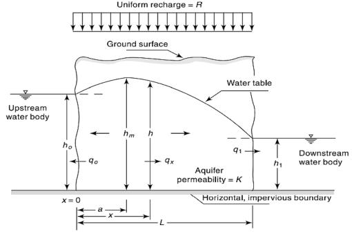
Fig. 2.10: One Dimensional Dupit Flow with Recharge
