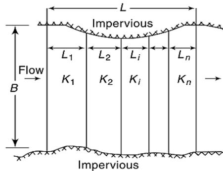
**Fig. 2.5(b)** Flow Normal to Stratification
