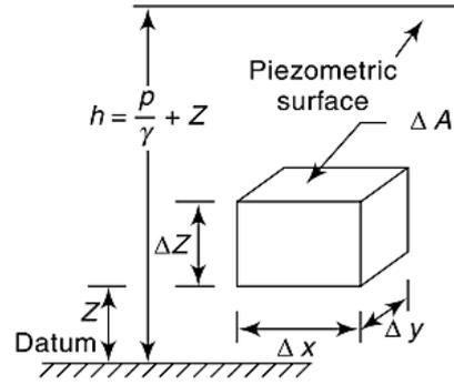
**Fig. 2.7 :** Volume element of a compressible aquifer
