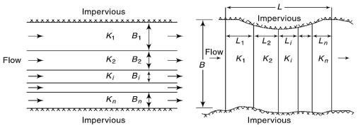
**Fig. 2.5(a)** Flow Parallel to Stratification
