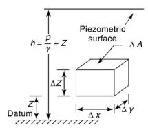
Fig. 2.7: Volume element of a compressible aquifer
