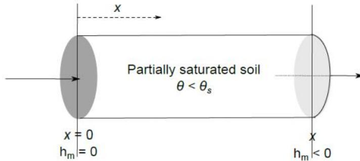
Fig. 13. Illustration of 1D steady-state flow through unsaturated soils
