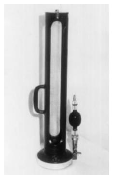
Figure (6.12) Calibrated vessel used with rubber balloon
