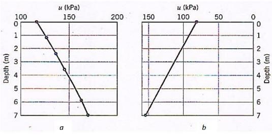
Figure 8.10 porewater pressure distributions (a) at front of wall and (b) at back of wall
