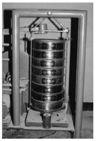
*Figure (5.1) A set of sieves for test in the laboratory*
