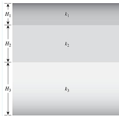
Figure (7.10) A layered soil profile
