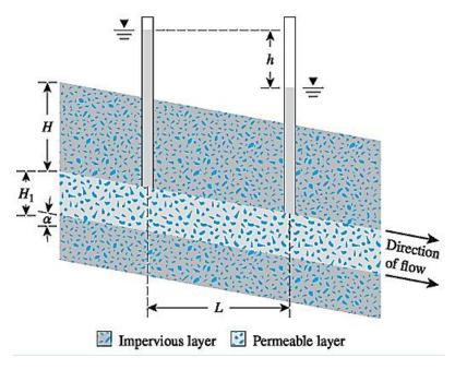
Figure 7.6 Flow through permeable layer
