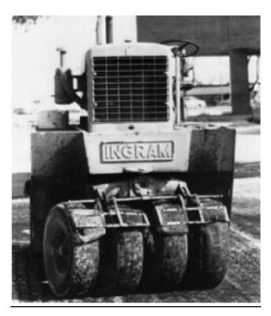
Figure (6.8) Pneumatic rubber-tired roller
