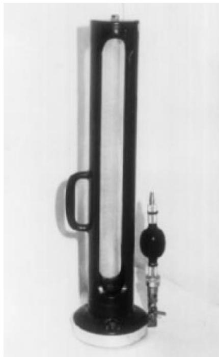
Figure (6.12) Calibrated vessel used with rubber balloon
