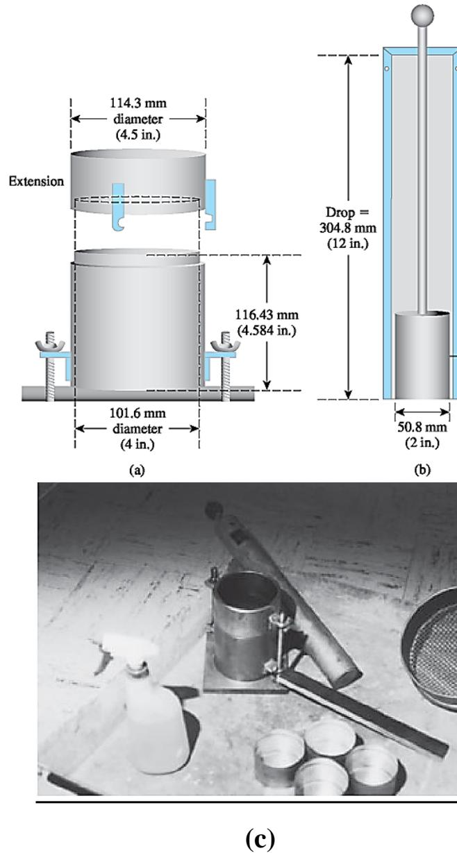
Figure 6.2 Standard Proctor test equipment: (a) mold; (b) hammer; (c) photograph of laboratory equipment used for test
