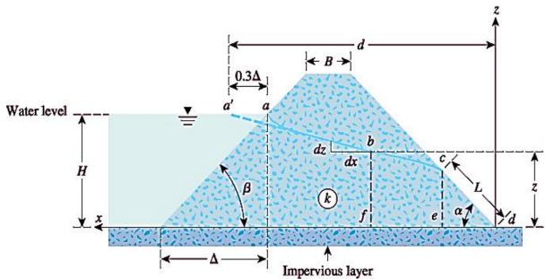
Figure (8.13) Flow through an earth dam constructed over an impervious base
