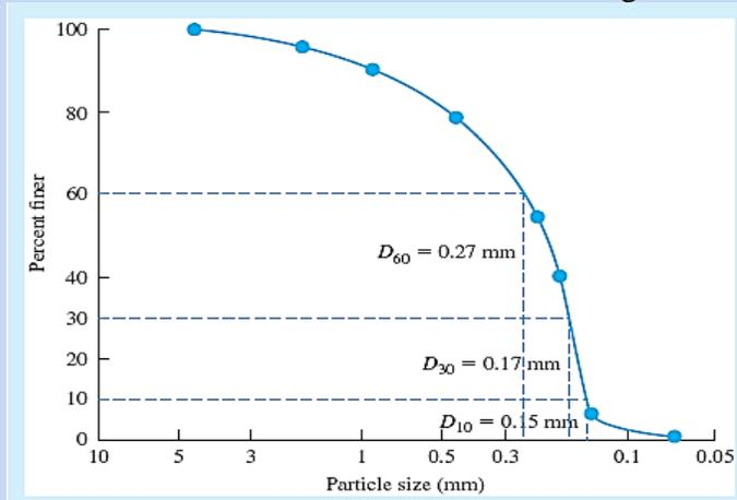
Figure (5.4) Particle-size distribution curve
