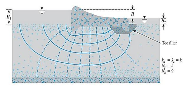
Figure 8.3 Flow net under a dam with toe filter
