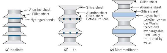
Structure of kaolinite, illite, and montmorillonite.
