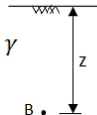
If water is seeping, the effective stress at any point in a soil mass will differ from that in the static case. It will increase or decrease, depending on the direction of seepage. The seepage force per unit volume is equal to:  $\gamma_w \cdot i$ . This force produces a stress with a soil mass at depth  $z$  equal to:  $\gamma_w \cdot i \cdot z$ . Thus, the effective stress will be:
