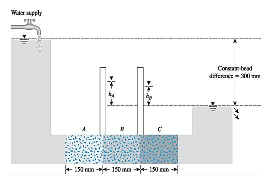
Figure (7.11) Three layers of soil in a tube 100 mm  $\times$  100 mm in cross section
