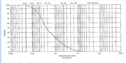
Figure (5.5) Grain-size Distribution curve for Example (5.4)
