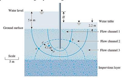
Figure 8.5 Flow net for seepage around a single row of sheet piles
