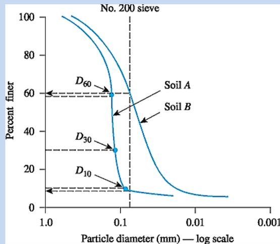
Figure (5.10) Particle size distribution of two soils
