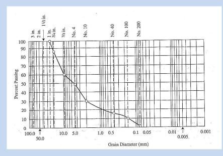
Figure (5.9) Grain-size Distribution curve for Example (5.6)
