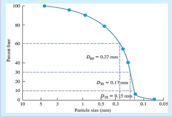
Figure (5.4) Particle-size distribution curve
