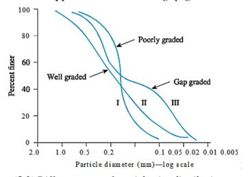
*Figure (5.3) Different types of particle-size distribution curves*
