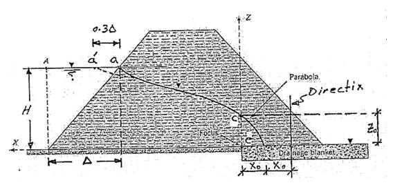
Figure (8.14) A horizontal drainage blanket at the toe of an earth dam
