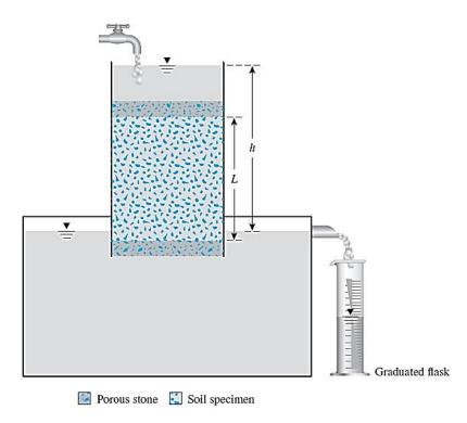
Figure (7.3) Constant-head permeability test
