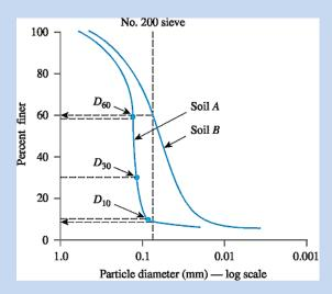
Figure (5.10) Particle –size distribution of two soils
