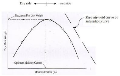
Figure 6.1 Principles of compaction
