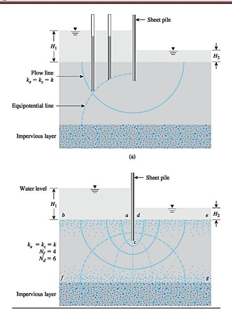
Figure 8.2 (a) Definition of flow lines and equipotential lines; (b) completed flow net
