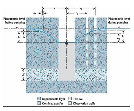
Figure (7.13) Pumping test from a well penetrating the full depth in a confined aquifer This gives the hydraulic conductivity in the direction of flow as
