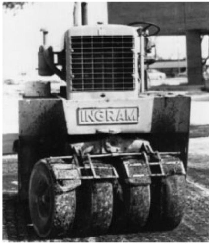
Figure (6.8) Pneumatic rubber-tired roller
