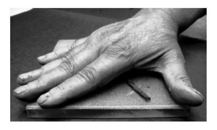
Figure (4.4) Rolling of soil mass on ground glass plate to determine plastic limit
