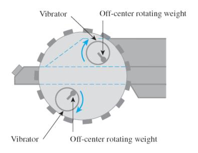
Figure (6.10) Principles of vibratory rollers
