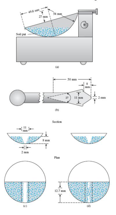
Figure (4.2) Liquid limit test: (a) Liquid limit device; (b) grooving tool; (c) soil pat befor test; (d) soil after test
