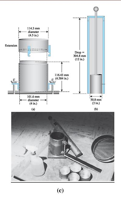
Figure 6.2 Standard Proctor test equipment: (a) mold; (b) hammer; (c) photograph of laboratory equipment used for test
