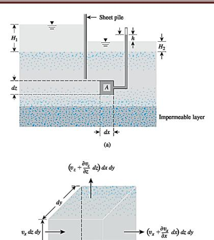
Figure 8.1 (a) Single-row sheet piles driven into permeable layer; (b) flow at A
