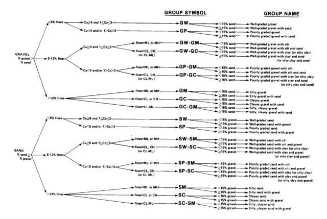
Figure (5.8) flow chart for classifying coarse -grained soils (More than 50% retained on No. 200 seive)
