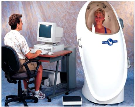
The BOD POD device estimates a person's body volume by measuring the space the body occupies while seated inside the chamber.
