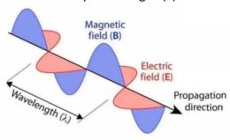
Electromagnetic radiation as a wave travels through space at the speed of light C which is 3\*10<sup>8</sup> m/s. Figure below gives an overview over the whole spectrum of electromagnetic waves.
