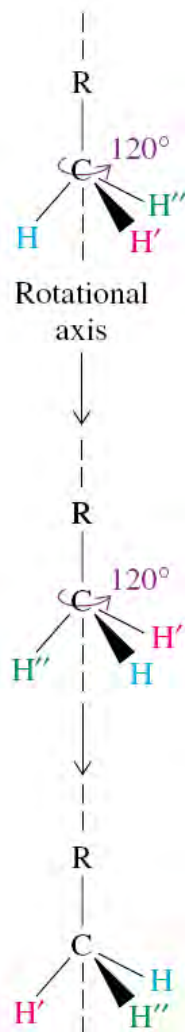
Figure 10-12 Rotation of a methyl group as a test of symmetry.
