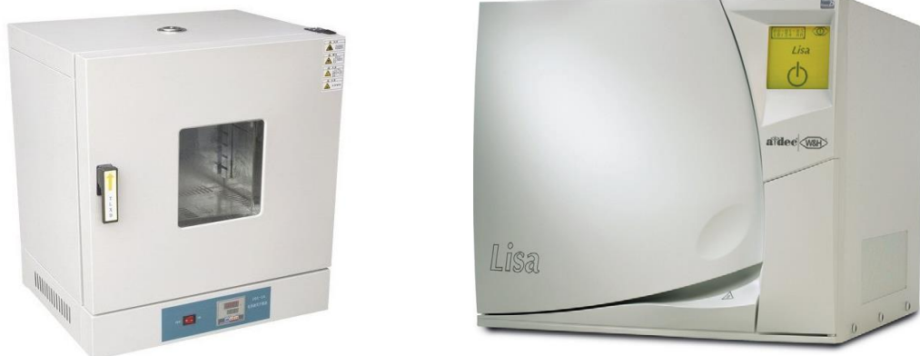
Figure 1 Sterilization with heat: Conventional oven (Left), Autoclave sterilizer (Right)
