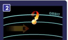
Pumping level is unstable, so the electron quickly jumps to a slightly lower energy level.
