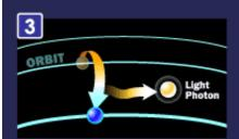
Electron relaxes to a lower energy state and releases a photon.
