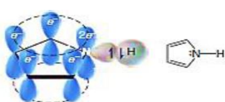
Figure 14.21 Pyrrole is aromatic but not basic. It does not have any unshared electron pairs. The electron pair on nitrogen is part of the aromatic system.
