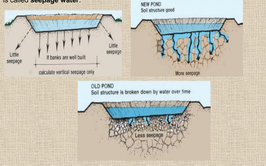
the rate of <u>seepage losses</u> in millimeters per day (mm/day) from various soil types (in the natural state) needed to calculate pond seepage losses over a period of time.
