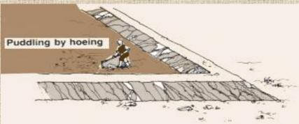
To calculate the amount of water needed for puddling multiply the pond area (in m<sup>2</sup>) by 0.3 m.
