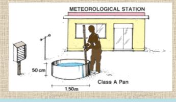
**Note**: water evaporates faster from a Class A Pan than from a large water surface such as a pond. When using Class A Pan evaporation rates you must multiply by a **correction factor** of 0.75 to better approximate evaporation losses
