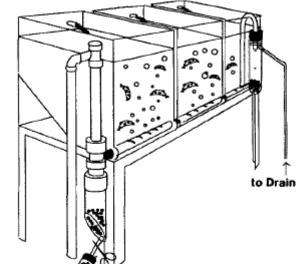
ig. 3. TUF Column attached to the first tank of the Guelph System.
