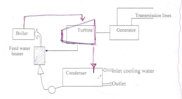
The figuer above shows a schematic diagram of a typical power plant using a Ranking energy conversion cycle.
