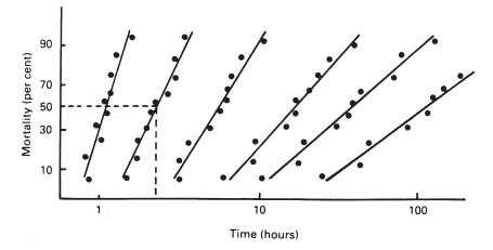
**Figure 4.1** Probit lines resulting from plots of cumulative percentage mortality in each test tank against time, using logarithmic-probability graph paper. The dotted lines show how median survival times are read from each line. Lines on the left are for the higher poison concentrations
