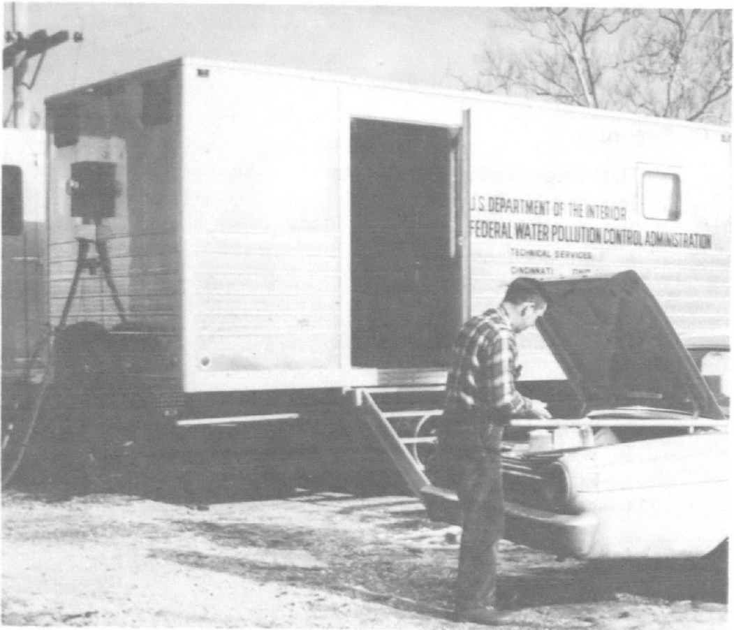
Figure 10. Mobile chemical and microbiological laboratories receiving samples near river bank.
