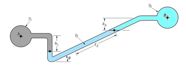
$$P_A + \gamma_1 h_1 - \gamma_2 l \sin \theta - \gamma_3 h_3 = P_B$$
