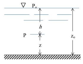
*Example 2.1* Determine the pressure of sea water at 10 m under sea level. Given the sea water density as 1020 kg/m<sup>3</sup>. Consider the value of atmospheric pressure as 101.3 kPa.
