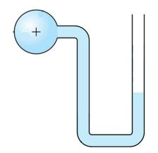
3- U-Tube Manometer with Multi-Liquids: It is U tube with using another liquid(s) of greater gravity. It is used for greater positive and negative pressure.
