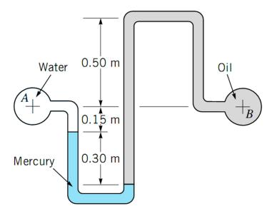
Example 2.5: For the inverted manometer shown in figure, if  $P_B$ - $P_A$ = 90 kPa, what must the height H be?
