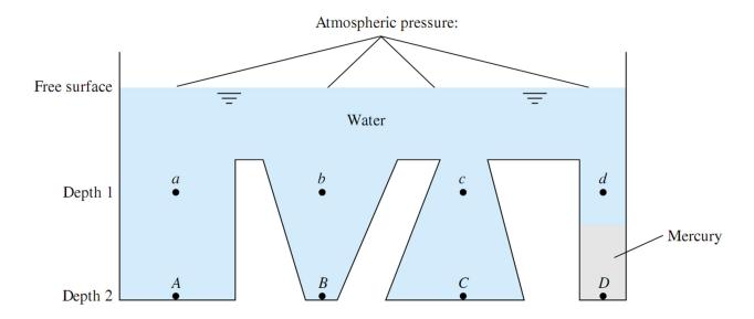
Points a, b, c, and d are at equal depths in water and therefore have identical pressures. Points A, B, and C are also at equal depths in water and have identical pressures higher than a, b, c, and d. Point D has a different pressure from A, B, and C because it is not connected to them by a water path.
