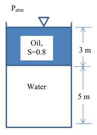
**Note:** Pressure doesn't vary horizontally, provided that the fluid is connected. To illustrate this statement, we may refer to the figure below.
