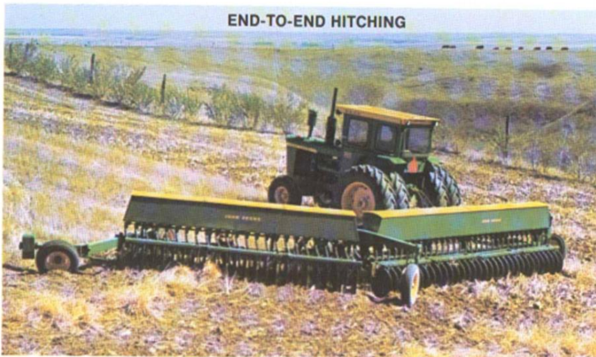
Fig. 36—End-to-End Hitching with Ball-and-Socket Coupling
