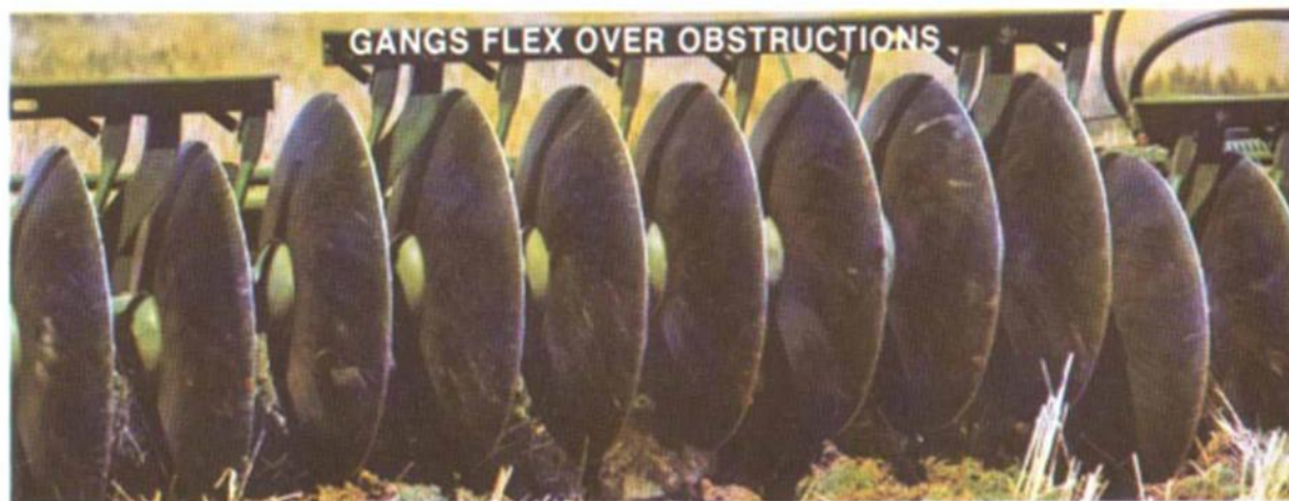
Fig. 8—Gangs Can Flex Over Obstructions
