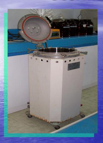
1- inside laboratory by using autoclave for 15 minutes
