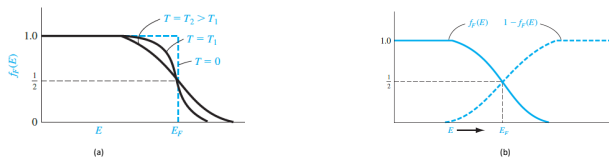
Figure: f_F(E) vs energy for different temperatures. (b) The probability functions f_F(E) and (1 - f_F(E)) .
