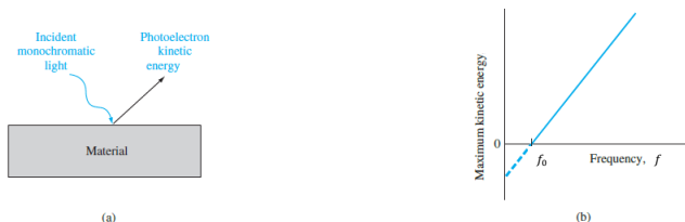
Figure: (a) Photoelectric effect. (b) Kinetic energy of the electrons versus frequency
